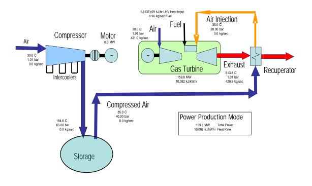
Figure 24: Schematic and Heat and Mass Balance for the CAES AI Plant Option Without Air Injection (Based on Performance of GE7241-FA-CT)
