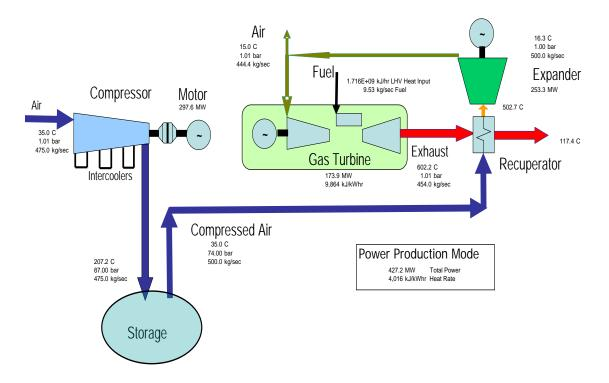
Figure 27: Schematic and Heat and Mass Balance for the CAES/Expander/Inlet Chilling Plant Option
