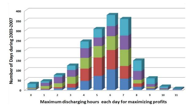
Figure 187: Anticipated operating hours for CAES unit with power ratio of 0.75 during 2003–2007
