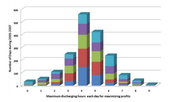
Figure 36: Anticipated operating hours for CAES unit with power ratio of 0.5 during 2003–2007
