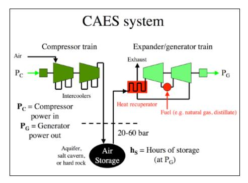
Figure 33: Typical CAES System Configuration (Succar, 2008)
