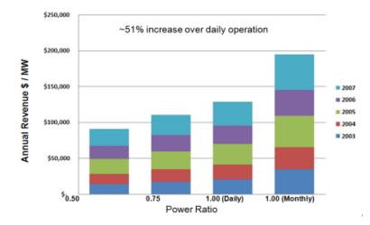
Figure 42: Expected net revenues from energy arbitrage for different power ratios with daily and monthly optimization
