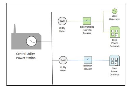
There is no standard, industry-accepted definition of a "microgrid" largely due to the many models and applications available. For the purposes of this study, a microgrid is defined as "a group of interconnected loads and distributed energy resources that form a single controllable entity capable of operating continuously in both grid-connected and islanded mode."
