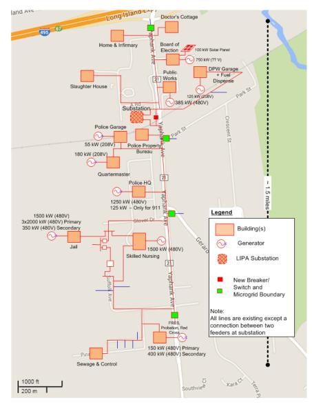
Figure D.1. Suffolk County One-line Interconnection Diagram
