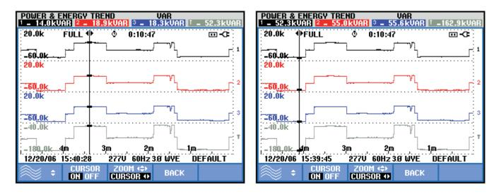
Fig. 6 Smart Energy Matrix supplies capacitive reactive power. The reactive load of the industrial facility changed from 109kVAr to 52kVAr. Fig. 7 Smart Energy Matrix supplies inductive reactive power. The reactive load of the industrial facility changed from 109kVAr to 163kVAr.
