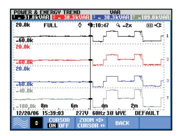
Fig. 5 Total reactive power before test = 109kVAr.
