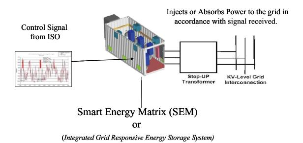
The Control Signal directs the system to inject or absorb power. Initially the system will respond to the variation in the grid frequency. Later the system may be configured to respond to a signal from the NYISO.
