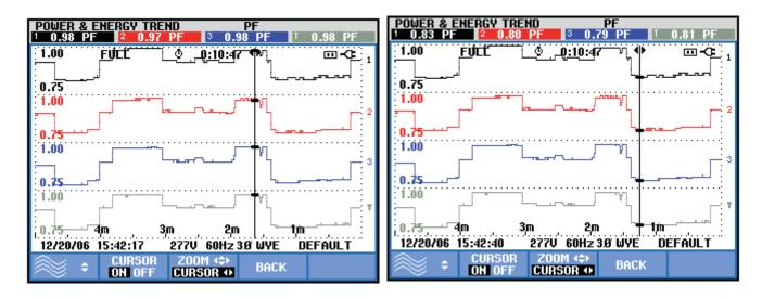
Fig. 3 Smart Energy Matrix supplies capacitive power. PF improved from 0.9 to 0.98 Fig. 4 Smart Energy Matrix supplies inductive power. PF of the industrial facility changed from 0.9 to 0.8
