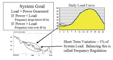
Figure 1 - Frequency regulation versus daily load changes
