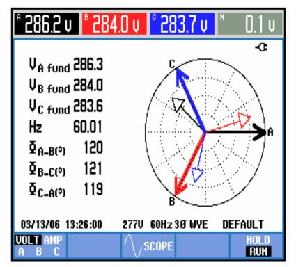
50KW discharge, -30KVAR, pf= -.742 Capacitive
