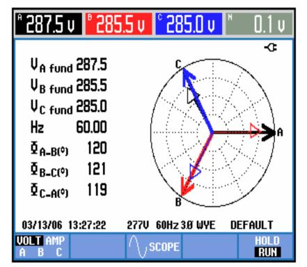
50KW Discharge, -50KVAR, pf= -0.534 Capacitive
