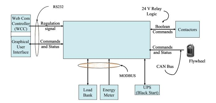
The main goal for the Master Controller is to send power commands to the load bank and flywheels to meet the overall power request for the system. It's secondary functions are state of health monitoring, and command / status processing.
