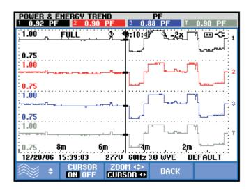
Fig. 2 Power Factor (PF) before test = 0.9.
