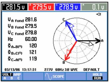
Phasor diagram at 60KW Charge (absorbing)
