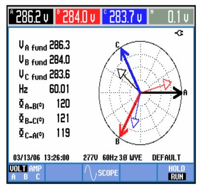
50KW discharge, -30KVAR, pf= -.742 Capacitive
