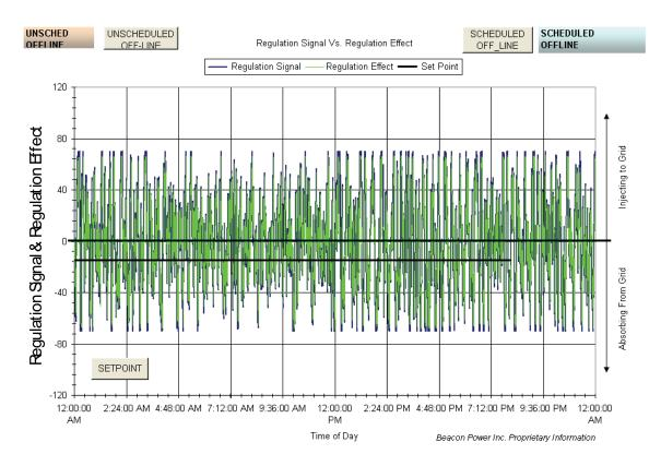
Figure 14 - Typical response generated from smoothed frequency signal
