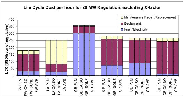
Figure 7: Comparison of the hourly LCC over the PJM, CAISO and ISONE regions shows little deviation in cost
