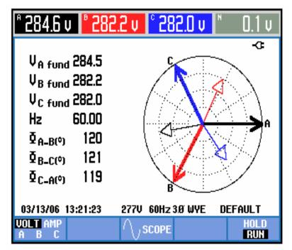
Discharge, voltage and current out of phase.
