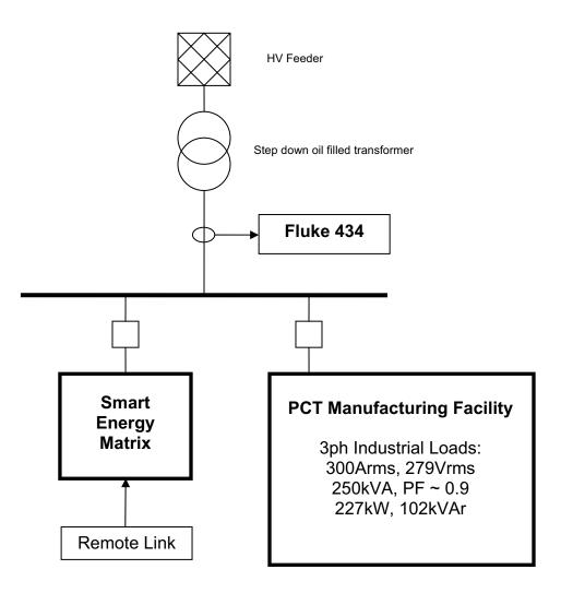
Fig. 1 Single line diagram of the test.
