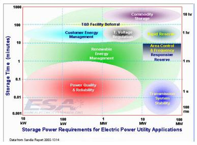
Figure 3. Storage Discharge Duration and Power Requirements for Applications
