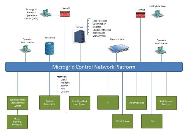
Figure 5-2. Conceptual microgrid control system architecture. (Adapted from Feasibility Study #49)
