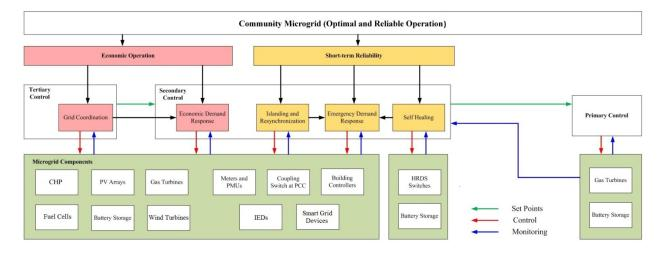
"In order to achieve the optimal economics, microgrids apply coordination with the utility grid and economic demand response in island mode. The short-term reliability at load points would consider microgrid islanding and resynchronization and apply emergency demand response and self-healing in the case of outages. Functionally, three control levels are applied to the community microgrid:
