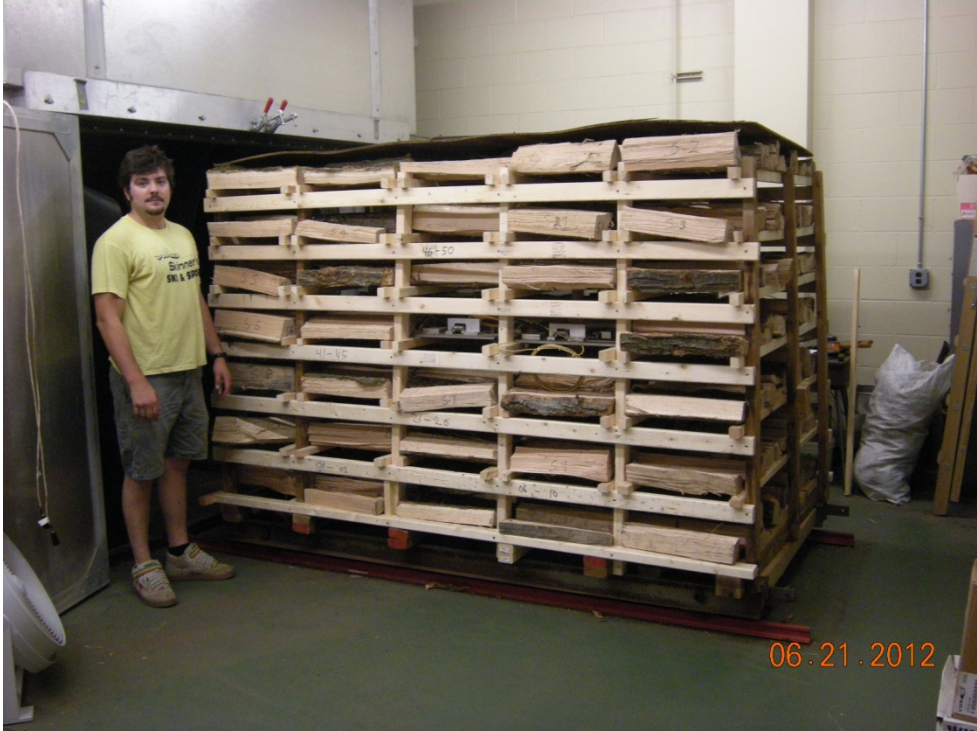
Figure 3 Red oak cordwood being loaded into lumber dry kiln
