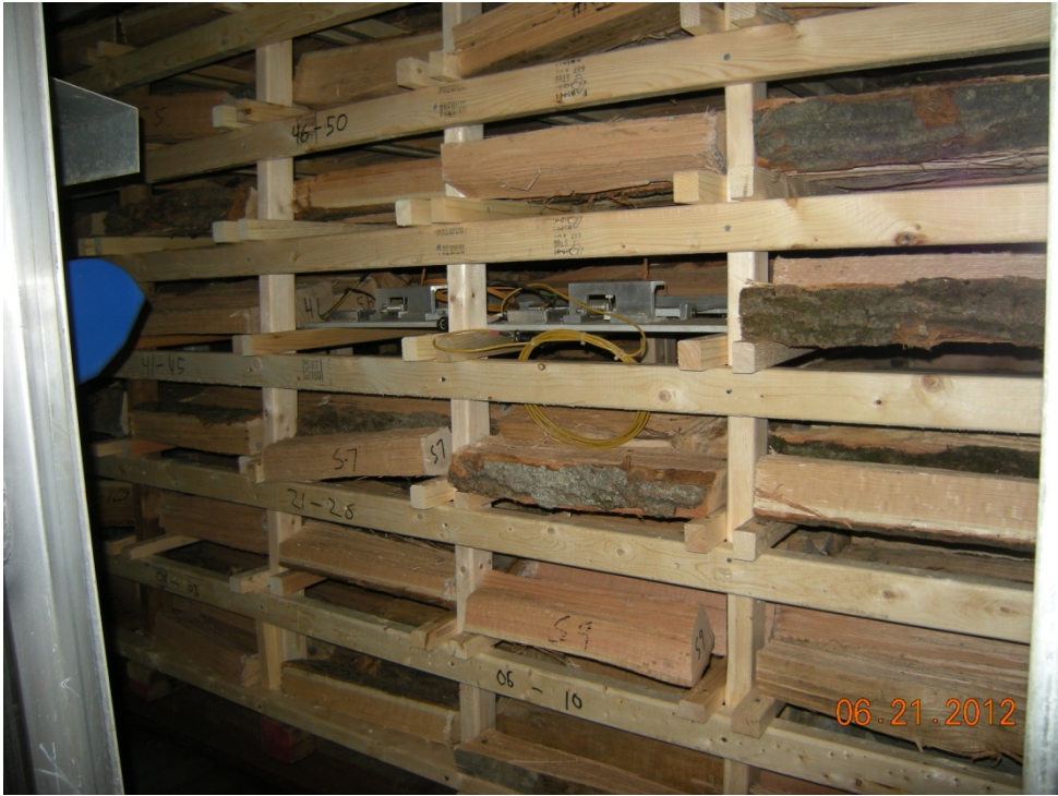
Figure 4. Red oak cordwood on racks in lumber dry kiln
