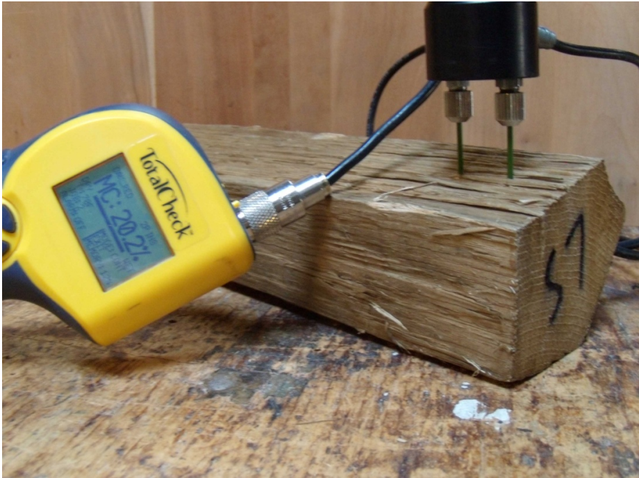
Figure 11. Core moisture determined with moisture meter (ex. 24.3% MC)
