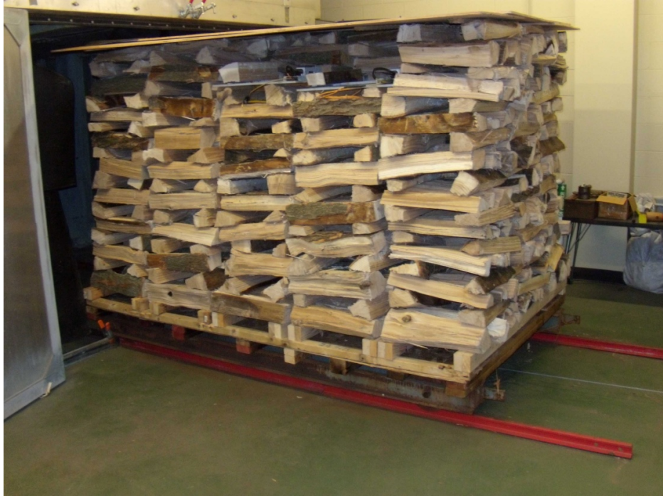
Figure 6. Red oak cordwood stacked crib-style for third kiln run
