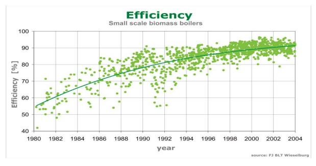
Figure 6. Efficiency improved from 55% to > 90% (based on LHV) over 25 years (Voglaur, 2005).
