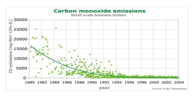
Figure 7. Carbon monoxide emissions drop from 15,000 to < 50 mg/m3 over 25 years (Voglaur, 2005).
