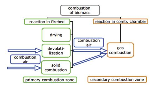
Figure 4. Process schematic of two stage combustion (NYSERDA, 2010).
