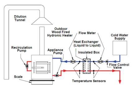
Note: Illustrated appliance pump location and flow path through the appliance are genaric and may vary based on the unit being tested.
