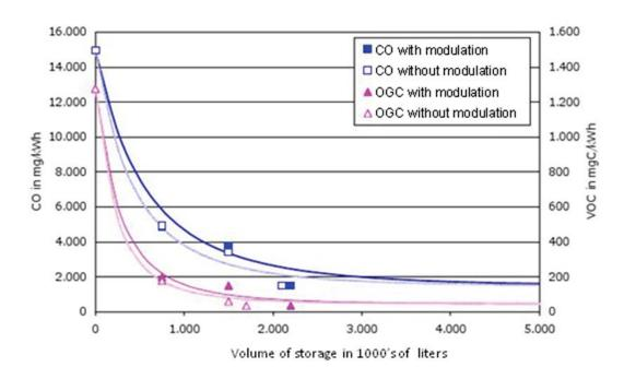
Figure 11. Emission reductions in CO and organic gases with thermal storage (Struschka et al., 2004).
