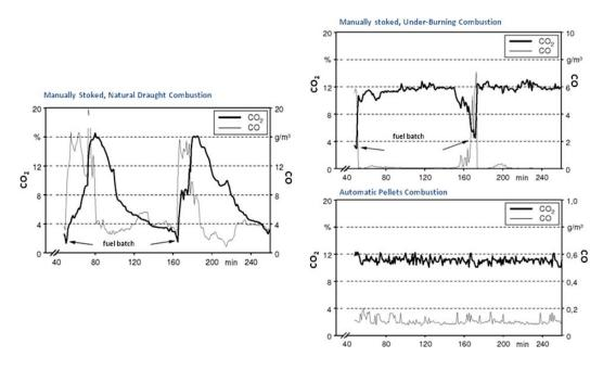
Figure 5. Comparisons of real-time CO/CO2 emissions for through combustion, two-stage split wood, and 2-stage pellet boiler combustion performance (Hartmann, 2003).
