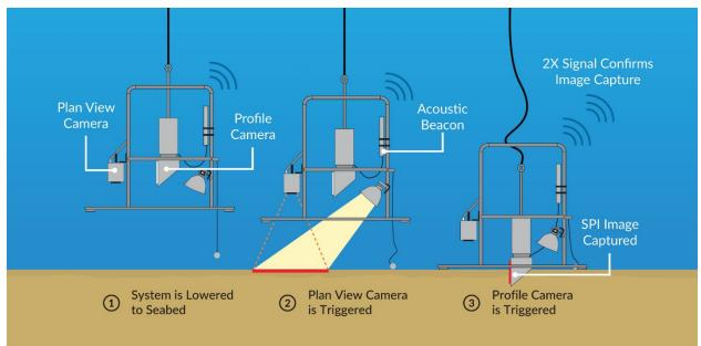
Figure 1. Schematic diagram of SPI/PV deployment
