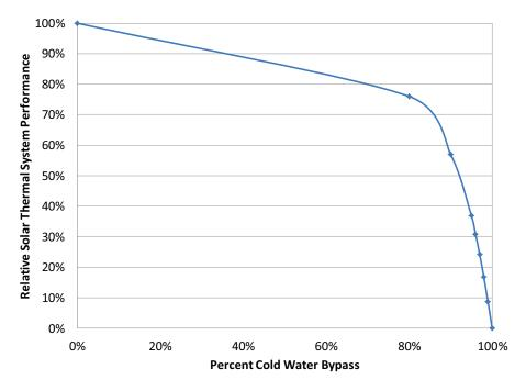
Figure 5: Simulated degradation of thermal energy production due to cold water bypass
