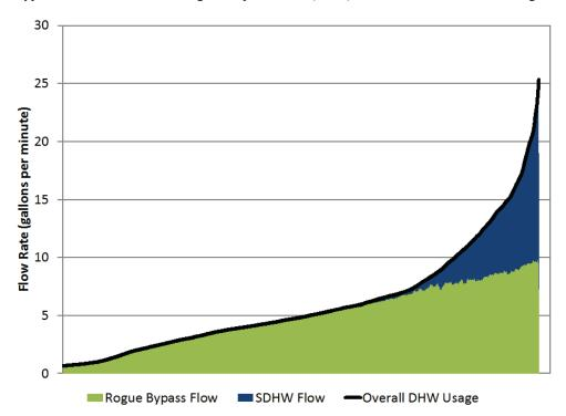
Figure S-3: One minute measurements of DHW usage, rogue bypass flow ( $F_{RB}$ ), and solar preheat tank flow ( $F_{CW}$ ), sorted from lowest usage to highest usage and presented to display contributions at given times 9
