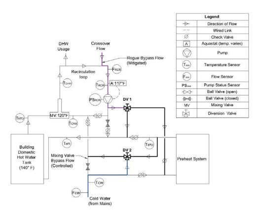
Figure 14: Modified schematic of SDHW system with proposed design solutions
