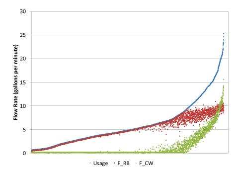
Figure S-3: One minute measurements of DHW usage, rogue bypass flow (F<sub>RB</sub>), and solar preheat tank flow (F<sub>CW</sub>), sorted from lowest usage to highest usage – unsmoothed (reference Figure S-3)
