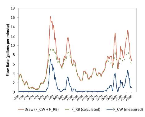
Figure 10: Typical daily profile of DHW usage, rogue bypass flow (F<sub>RB</sub>), and solar preheat tank flow (F<sub>CW</sub>)
