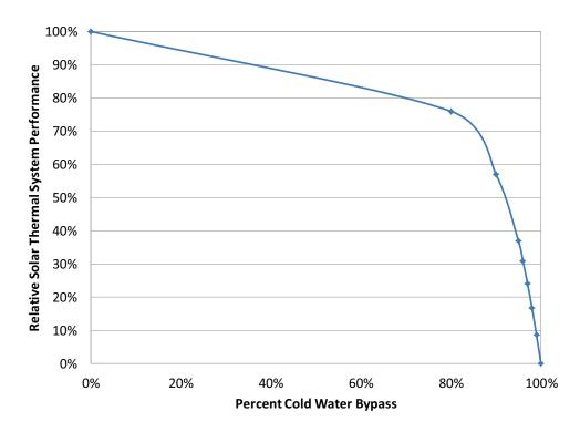
Figure S-1: The negative effect of cold water bypass on solar thermal system performance<sup>5</sup>
