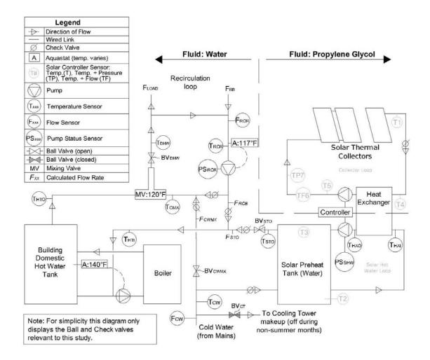
Figure 3: Schematic of solar system with sensor locations
