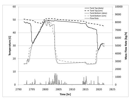
Figure 17: "Calibrated" Daily Solar Preheat Tank Temperature Profile (Measured and Simulated)
