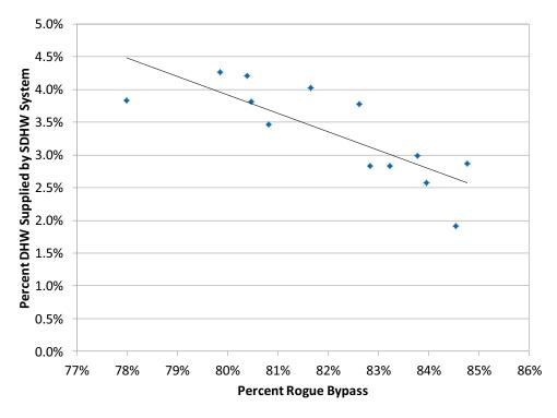
Figure 9: Correlation between weekly averages of % rogue bypass % DHW supplied by the SDHW system (by volume)
