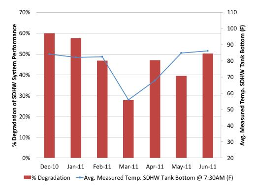
Figure 4: Negative impact to system performance correlated with reduced flow through solar preheat tanks
