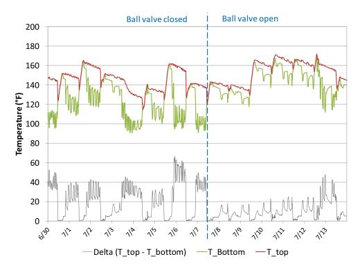
Figure 7: Temperatures at top and bottom of solar preheat tank with ball valve open (6/30 to 7/6) and closed (7/7 to 7/13)
