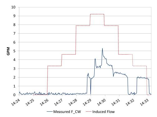
Figure 8: Comparison of measured vs. induced flow rates in the absence of mixing valve bypass
