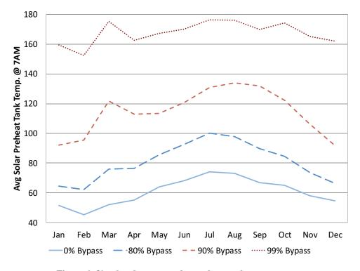
Figure 6: Simulated average solar preheat tank temperatures for increasing percentages of net cold water bypass
