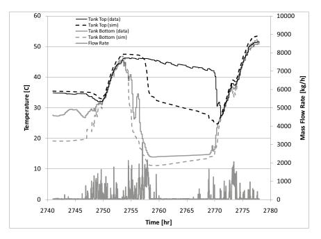
Figure 16: Typical Daily Solar Preheat Tank Temperature Profile (Measured and Simulated)
