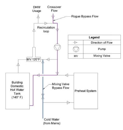
Figure 2: Two paths for cold water bypass
