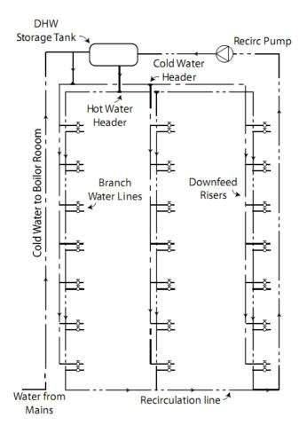
Figure 12: Example schematic of riser and recirculation loop configuration
