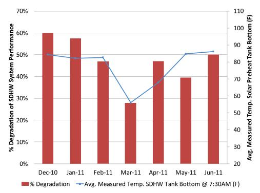
Figure S-2: Monthly average morning tank temperature and monthly total percent system degradation<sup>8</sup>
