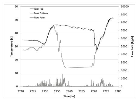
Figure 15: Typical Daily Solar Preheat Tank Temperature Profile (Measured Data)
