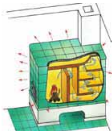
Figure 2-10 Functional principle of a tiled base stove (Kachelofenbauerinnung 2007)
