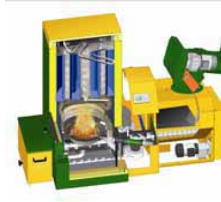
Figure ES-6 Underfeed burner or wood chips and pellets (KWB 2007)
