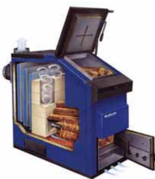
Figure 2-21 Under-burning boiler with induced draught, flue gas exit sideways(Buderus 2005)
