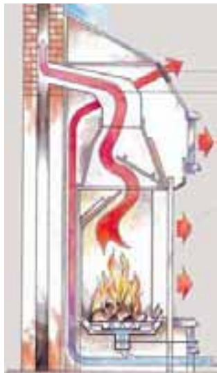
Figure 2-8 Functional principle of a log wood stove (Westfeuer 2005)
