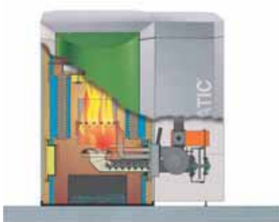
Figure 2-18 Underfeed boiler (Guntamatic 2007)
