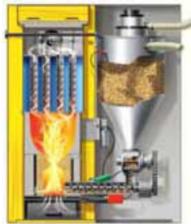
Figure 2-19 Horizontal feed boiler (Hargassner 2005)
