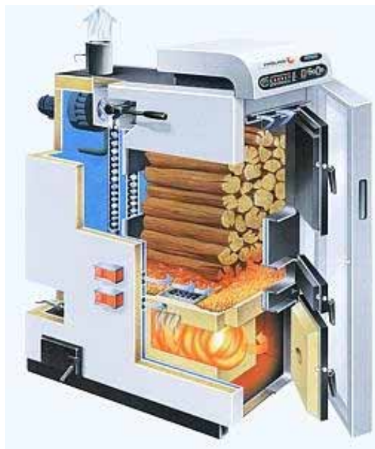
Figure 2-22 Under-burning boiler with induced draught, vertical flue gas exit (Froeling 2005)
