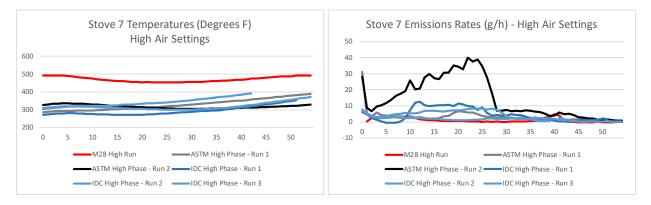
As shown in that figure, the temperature in the M28 high-fire run started out 180°F higher than the highest temperature at the beginning of the high-fire phases of the IDC runs and remained at least 100°F higher than in all IDC runs during the first 30 minutes of the run when most emissions occurred. This may at least partially explain the lower emissions rates for that portion of the M28 run, as shown in the second graph in that figure.
