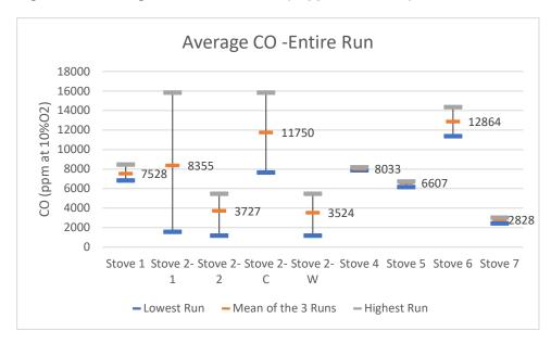
Figure 102. Average CO Concentration (in ppm at 10% O<sub>2</sub>)—Entire IDC Runs
