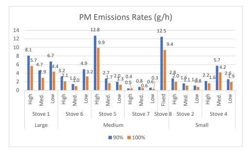
Figure 76. PM Emission Rates for 90% and 100% Combustion in M28 and ASTM 3053-17 Runs M28 Runs
