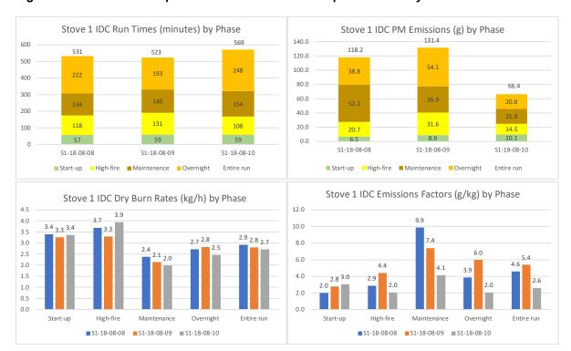
Figure 109. Stove 1—Comparison of Metrics for IDC Replicate Runs by Phase
