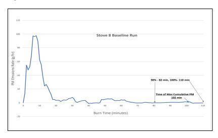
Note that the scales in the Figure 74 graphs are very different. Stove 1, the only large stove in this group, and stove 8, the fixed-air setting stove, had a considerably higher peak PM emission rate than the other stoves, while the instantaneous emission rates for stove 7, the stove with hybrid controls, were the lowest for all burn levels.
