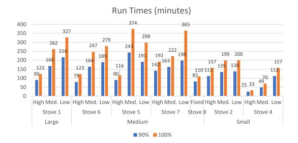
Figure 67. Method 28 Run Times at 90% and 100% Fuel Consumption
