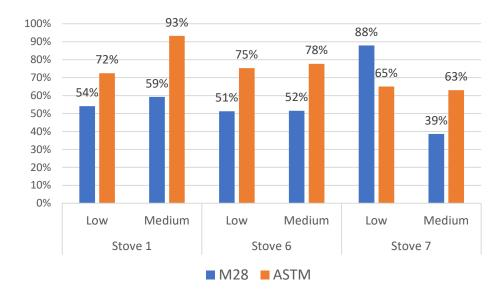
Figure 101. Percent Difference Between PM Emissions Rates (ER) at 100% and 90% Load Combustion in ASTM 3053-17 and M28 Medium- and Low-Air Runs
