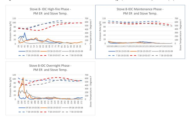
Figure 127. Stove 8—IDC Run Profiles—PM Emissions Rate (g/h) and Stove Temperature (°F)
