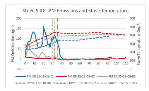
Figure 88. Stoves 5 and 6 High-Fire Phase PM Emissions and Stove Temperature Profiles
