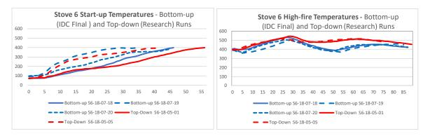
Temperatures in the start-up phase of the bottom-up runs tended to be higher than those in the top-down runs. The temperature difference was most notable in the runs for stove 2 and 5. As shown in Figure 4-11, the higher bottom-up temperatures were, in most cases, associated with higher burn rates and lower run times in the start-up phase.
