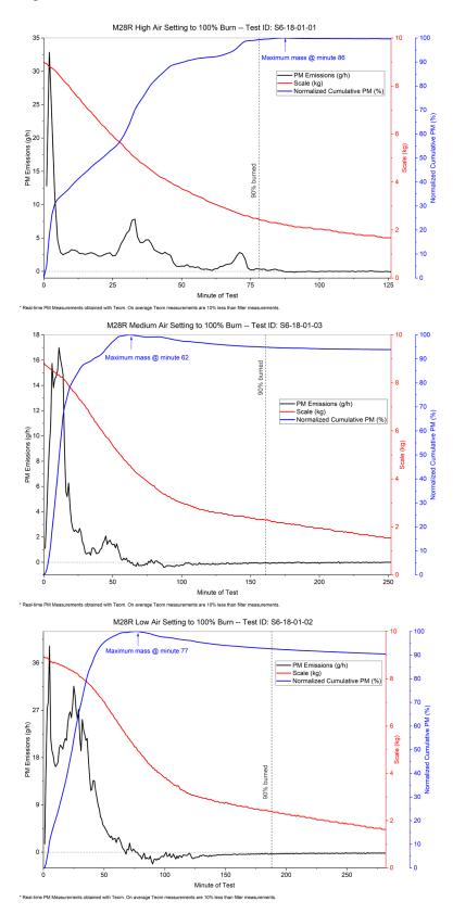
Instantaneous emissions were highest in the first few minutes of all three runs. The maximum instantaneous rate was 32.9 g/h at minute 2 of the high-burn run, 17.0 g/h at minute 11 of the medium run, and 39.2 g/h at minute 5 of the low run. In the high-burn run, the instantaneous PM emission rate dropped to below 4 g/h at minute 5 and were then above 4 g/h for an 11-minute period beginning at minute 38.
