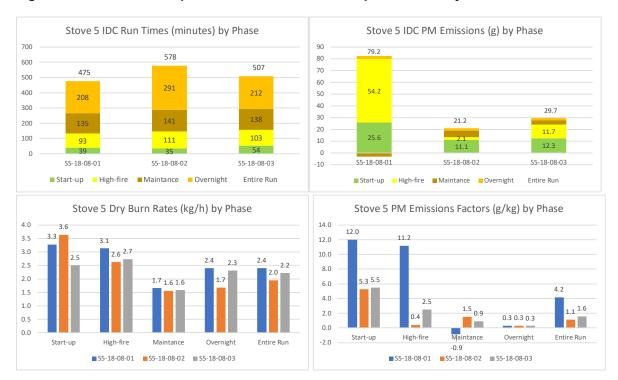
Figure 119. Stove 5—Comparison of Metrics for IDC Replicate Runs by Phase
