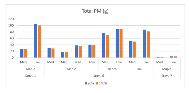
Figure 73. PM Emissions (g) in ASTM 3053-17 Low and Medium Runs at 90% and 100% Combustion
