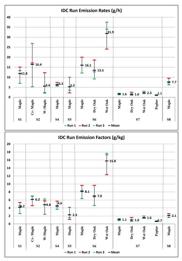
Figure 128. IDC Run Emission Rates (g/h) and Emission Factors (g/kg) by Stove and Fuel
