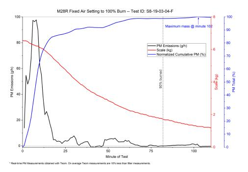
The maximum instantaneous emissions in the stove 8 M28 run, 97.8 g/h, occurred at minute 8 of the run. were much lower than in the other stoves. After the initial peak, the PM ER decreased to a baseline level at minute 17 that continued for the remainder of the run. At the point, 84% of total PM emissions had occurred and 18% of the fuel load had been consumed.
