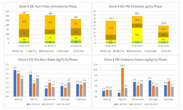
Figure 116. Stove 4—Comparison of Metrics for IDC Replicate Runs by Phase
