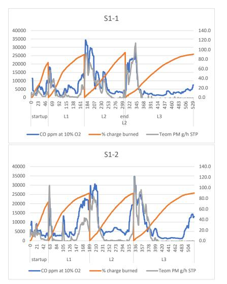
Figure 106. PM and CO Emissions Profiles and Percent of Load Combusted
