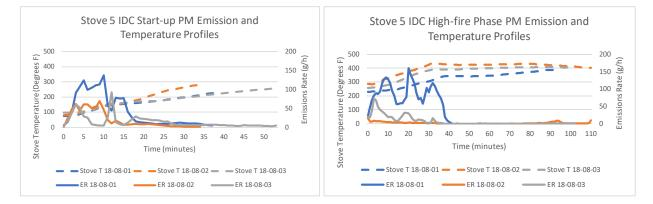
Stove temperatures were very low for most of the start-up phases of all runs. At those temperatures, the non-catalytic controls may not have been operable, so the stove would have been burning virtually uncontrolled during that period. However, because the temperatures were similar in the three runs during the early part of the start-up when most of the significant emissions occurred, that variable does not explain inter-run differences in that phase.
