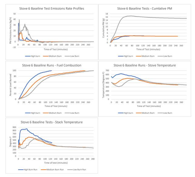
As shown Figure 33, the stove and stack temperatures were considerably higher and the burn rate faster in the high-burn run than the other runs. The low-air run fuel combustion curve and secondary emission peaks are consistent with a delayed light-off of the fuel load. The stove and stacks temperatures in that run were considerably lower than in the other runs throughout the period of significant PM emissions.
