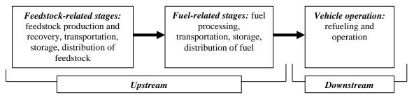
Figure 4-9. Components of a Total Fuel-Cycle from Winebrake, Wang, et al. (2001).
