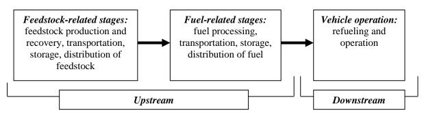
Figure ES-11. Components of a Total Fuel-Cycle from Winebrake, Wang, et al. (2001).
