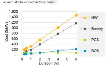
Figure 3: Cost by duration (2019, Li-Ion, utility-scale, hardware components)<sup>a</sup>
