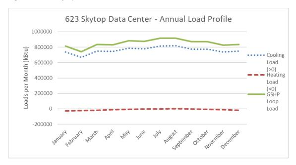
Note that the GSHP load is more than the cooling load because it includes the heat of the heat pump compressor, which the geothermal loop must alleviate.
