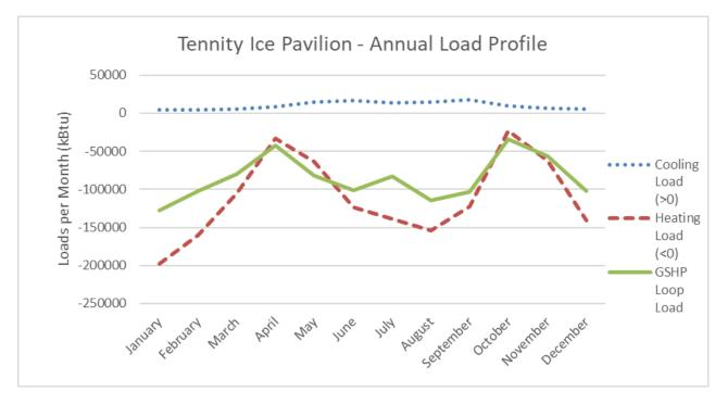
Note the load profile does not include the cooling for the ice.
