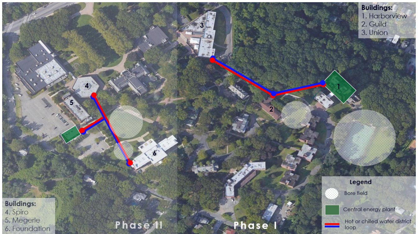
Figure 6. Two-Phase District Geothermal Concept
