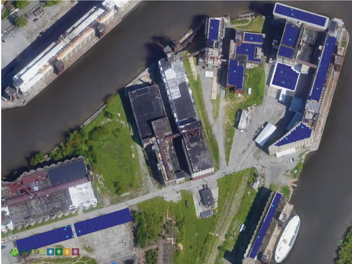
Figure 8. Solar PV Array Siting
