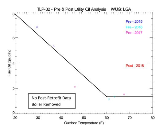
Figure 5. Trend of Oil Use with Outdoor Temperature Data, Using Fuel Delivery Logs from Pre, and Post-Retrofit Periods
