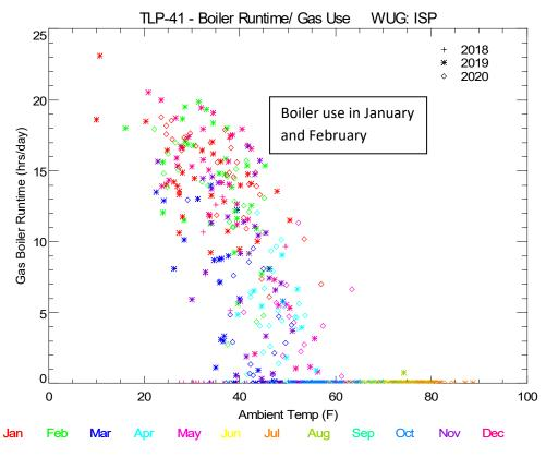
Figure 5. Daily Boiler Runtime versus Outdoor Temperature
