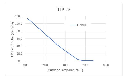
Figure 8. Trend of POST-Retrofit Electric Use with Outdoor Temperature for Bin Analysis
