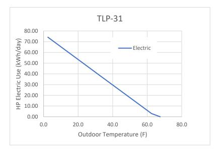
Figure 8. Trend of POST-Retrofit Electric Use with Outdoor Temperature for Bin Analysis
