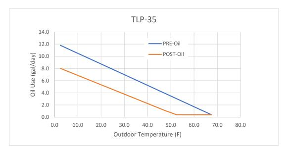
Figure 7. Trend of PRE- and POST-Retrofit Oil Use with Outdoor Temperature for Bin Analysis
