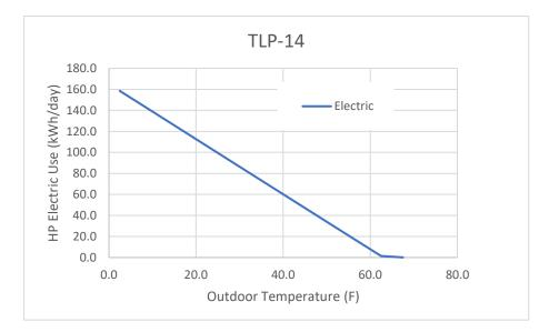
Figure 7. Trend of POST-Retrofit Electric Use with Outdoor Temperature for Bin Analysis
