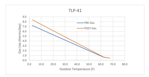
Figure 7. Trend of PRE- and POST-Retrofit Gas Use with Outdoor Temperature for Bin Analysis
