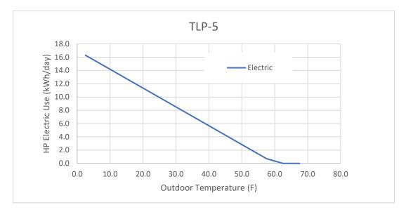
Figure 8. Trend of POST-Retrofit Electric Use with Outdoor Temperature for Bin Analysis
