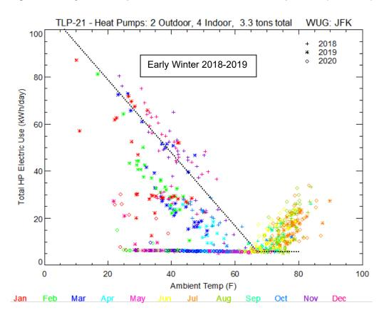
Figure 12. Daily Heat Pump Electric Use versus Outdoor Temperature (from JFK) at S21
