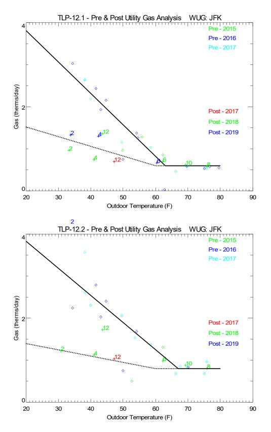
Figure 5. Trend of Gas Use With Outdoor Temperature Data, Using Fuel Delivery Logs from Pre, and Post-Retrofit Periods
