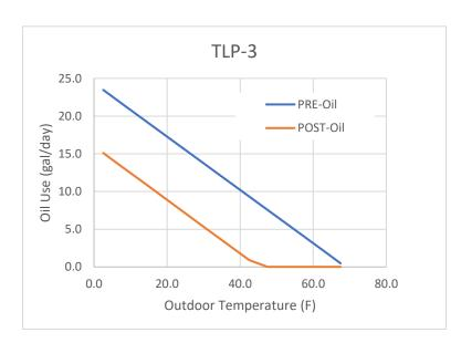
Figure 7. Trend of PRE- and POST-Retrofit Oil Use with Outdoor Temperature for Bin Analysis
