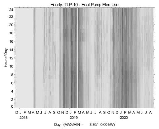
Figure 2. Shade Plot of Total Heat Pump Power
