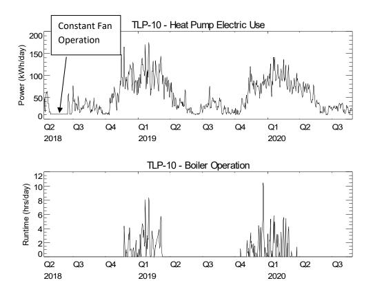
Figure 3. Plot of Daily Total HP Electric Use (and Daily Boiler Operation)
