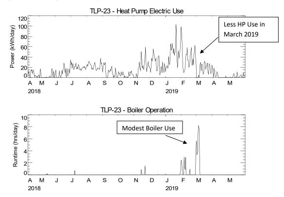
Figure 3. Plot of Daily Total HP Electric Use (and Boiler Operation)
