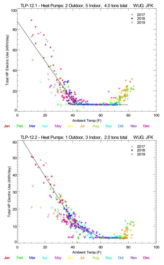
*Figure 4. Daily Heat Pump Electric Use versus Outdoor Temperature*
