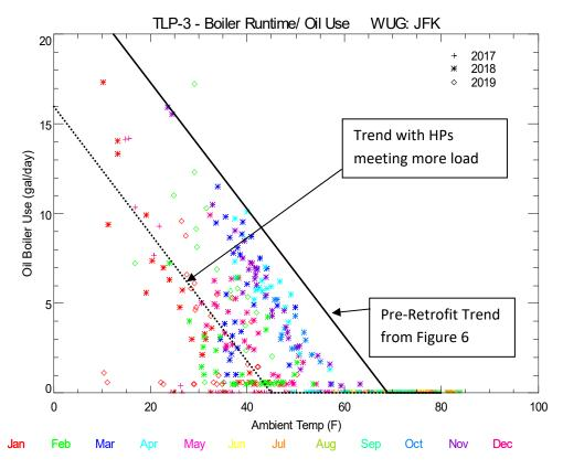
Figure 5. Daily Oil Use versus Outdoor Temperature (from JFK). Oil Use determined from Boiler Runtime.
