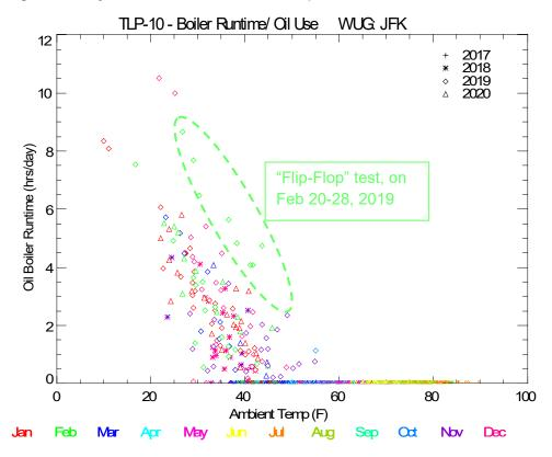
Figure 9. Daily Oil Use versus Outdoor Temperature at S10
