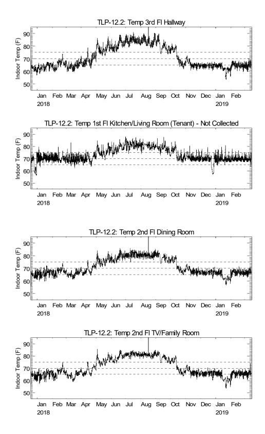
Figure 11. Plot of Space Temperatures at Various Indoor Locations for TLP12.2
