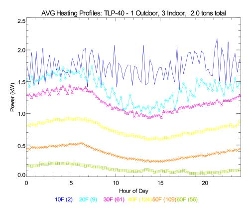
Figure 8. Heat Pump Demand Profile Across the Day – Averaged for Various Outdoor Temperature Bins (Heating)
