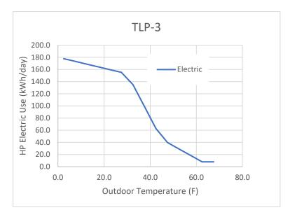
Figure 8. Trend of POST-Retrofit Electric Use with Outdoor Temperature for Bin Analysis
