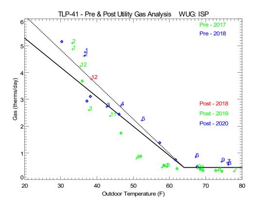
Figure 6. Trend of Gas Use with Outdoor Temperature Data, Using Fuel Delivery Logs from Pre- and Post-Retrofit Periods
