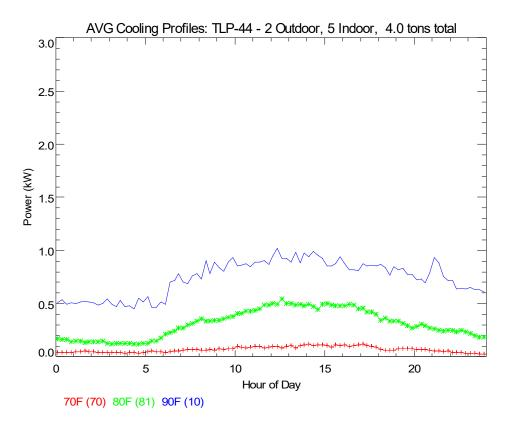
Figure 9. Heat Pump Demand Profile Across the Day – Averaged for Various Outdoor Temperature Bins (Cooling)
