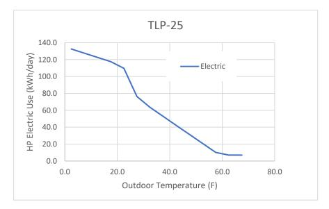
Figure 7. Trend of POST-Retrofit Electric Use with Outdoor Temperature for Bin Analysis
