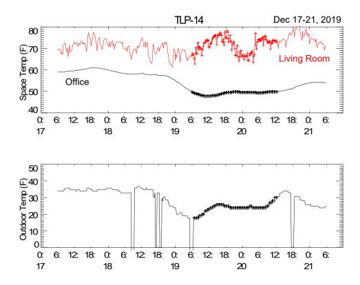
Figure 15. Period When Space Temperatures Dipped Below 50°F in the Heating Season at S14
