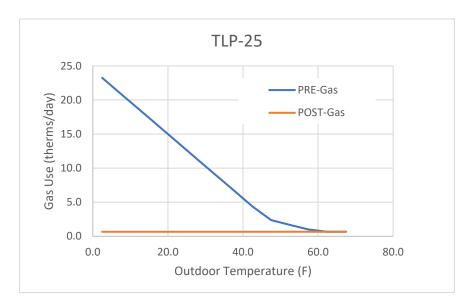
Figure 6. Trend of PRE- and POST-Retrofit Gas Use With Outdoor Temperature for Bin Analysis
