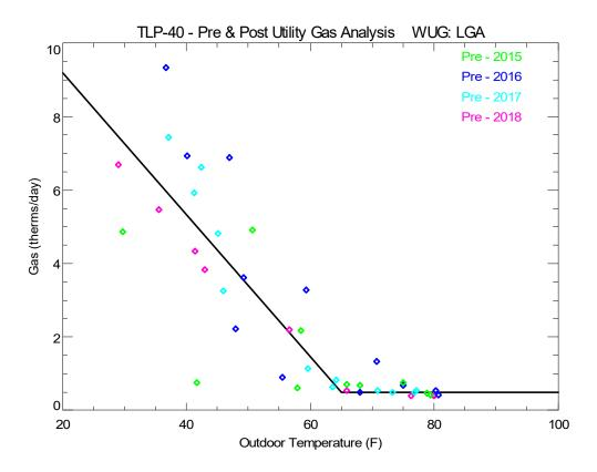
Figure 5. Trend of Gas Use with Outdoor Temperature Data, Using Fuel Delivery Logs from Pre- and Post-Retrofit Periods
