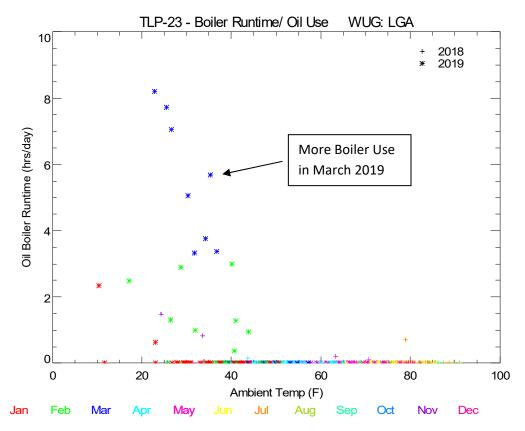
Figure 5. Daily Boiler Runtime versus Outdoor Temperature (from LGA)
