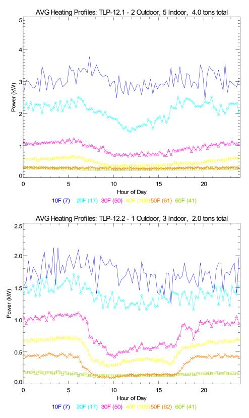
Figure 8. Heat Pump Demand Profile Across the Day – Averaged for Various Outdoor Temperature Bins (Heating)
