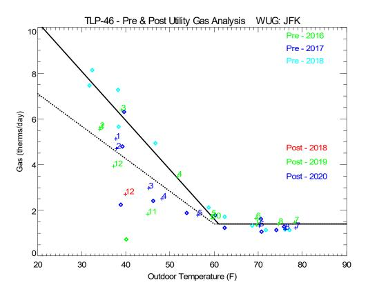
Figure 5. Trend of Gas Use with Outdoor Temperature Data, Using Fuel Delivery Logs from Pre, and Post-Retrofit Periods
