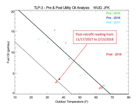
Figure 6. Trend of Oil Use With Outdoor Temperature Data, Using Fuel Delivery Logs from Pre, and Post-Retrofit Periods
