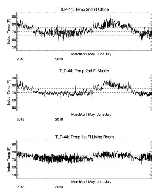
Figure 10. Plot of Space Temperatures at Various Indoor Locations
