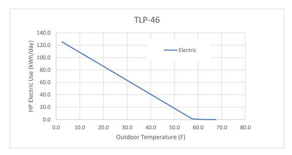
Figure 7. Trend of POST-Retrofit Electric Use with Outdoor Temperature for Bin Analysis
