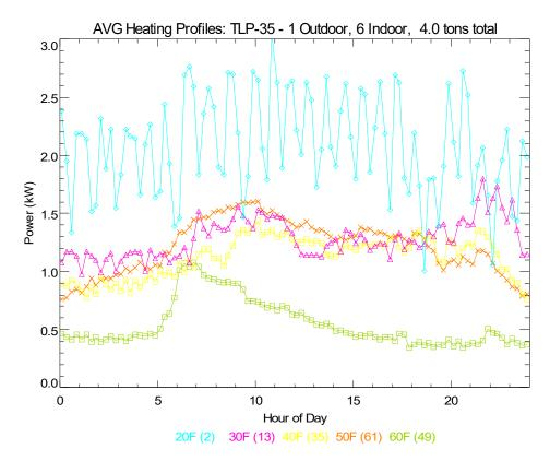
Figure 9. Heat Pump Demand Profile Across the Day – Averaged for Various Outdoor Temperature Bins (Heating)
