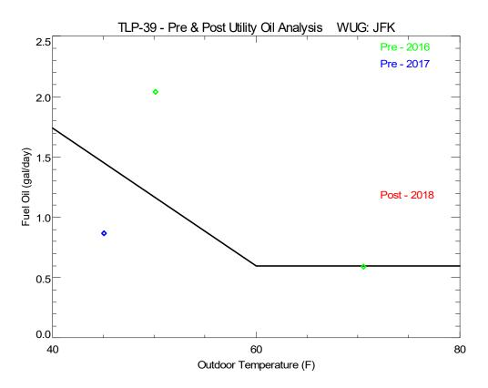
Figure 5. Trend of Oil Use with Outdoor Temperature Data, Using Fuel Delivery Logs from Pre, and Post-Retrofit Periods
