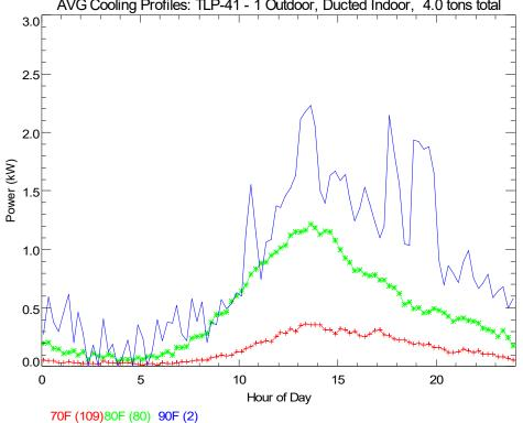
AVG Cooling Profiles: TLP-41 - 1 Outdoor, Ducted Indoor, 4.0 tons total
