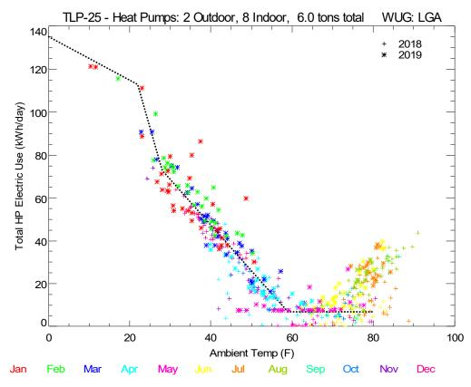
Figure 4. Daily Heat Pump Electric Use versus Outdoor Temperature
