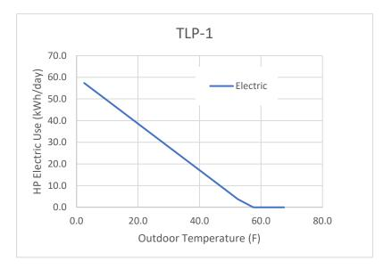
Figure 7. Trend of POST-Retrofit Electric Use with Outdoor Temperature for Bin Analysis
