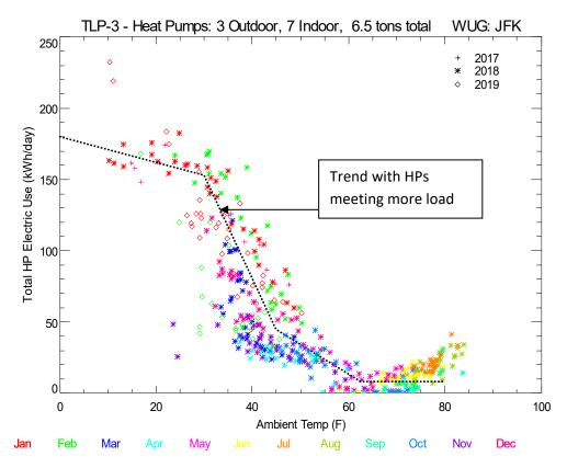
Figure 4. Daily Heat Pump Electric Use versus Outdoor Temperature (from JFK)
