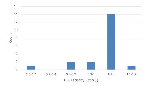
Figure 4. Distribution of Heat Pump H-C Capacity Ratio (QH5\_max per Nominal Cooling)
