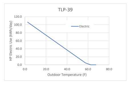
Figure 7. Trend of POST-Retrofit Electric Use with Outdoor Temperature for Bin Analysis
