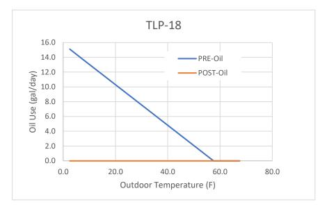
Figure 6. Trend of PRE- and POST-Retrofit Oil Use with Outdoor Temperature for Bin Analysis
