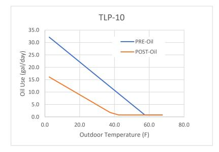
Figure 7. Trend of PRE- and POST-Retrofit Oil Use With Outdoor Temperature for Bin Analysis
