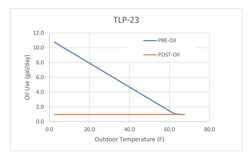
Figure 7. Trend of PRE- and POST-Retrofit Oil Use with Outdoor Temperature for Bin Analysis
