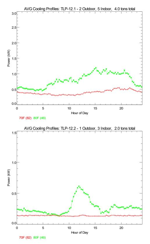
*Figure 9. Heat Pump Demand Profile Across the Day – Averaged for Various Outdoor Temperature Bins (Cooling)*
