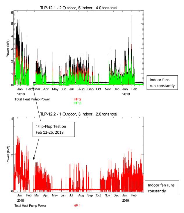
Figure 1. Plot of Power Use for All Heat Pumps at Site
