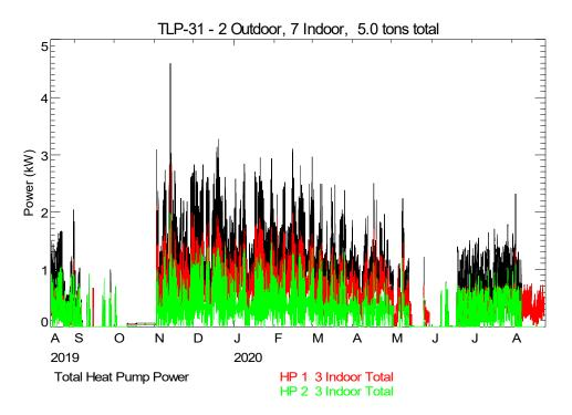
Figure 1. Plot of Power Use for All Heat Pumps at Site
