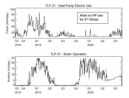
Figure 11. Plot of Daily Total Heat Pump Electric Use and Daily Boiler Operation at S21
