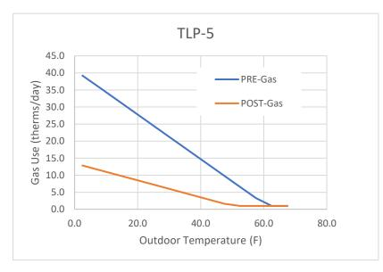
Figure 6. Trend of PRE- and POST-Retrofit Gas Use with Outdoor Temperature for Bin Analysis
