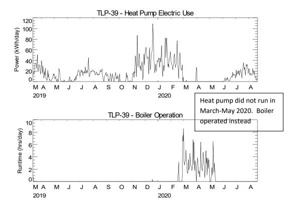
Figure 3. Plot of Daily Total HP Electric Use (and boiler runtime)
