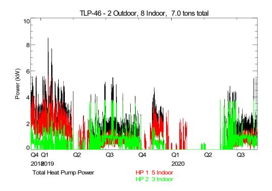
Figure 1. Plot of Power Use for All Heat Pumps at Site
