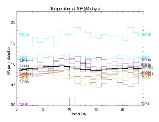
Figure 19. Normalized Demand Profiles for all Sites Combined at an Outdoor Temperature of 10°F
