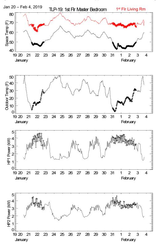
Figure 17. Periods When Space Temperatures Dipped Below 50°F in the Heating Season at S19
