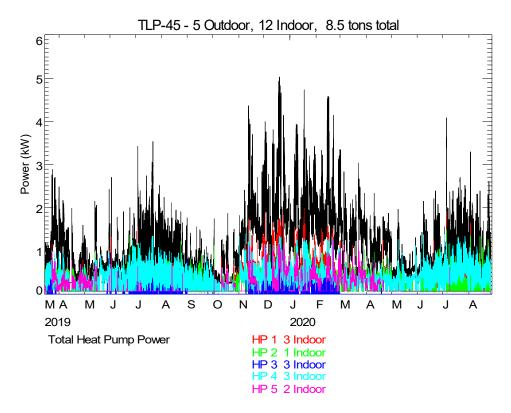
Figure 1. Plot of Power Use for All Heat Pumps at Site
