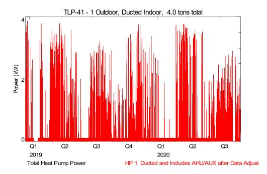
Figure 1. Plot of Power Use for All Heat Pumps at Site
