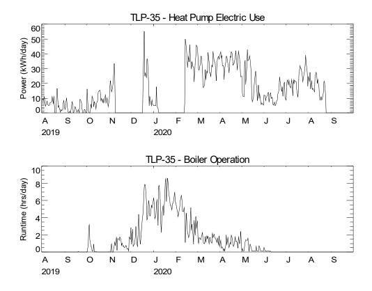
Figure 3. Plot of Daily Total HP Electric Use (and boiler runtime)
