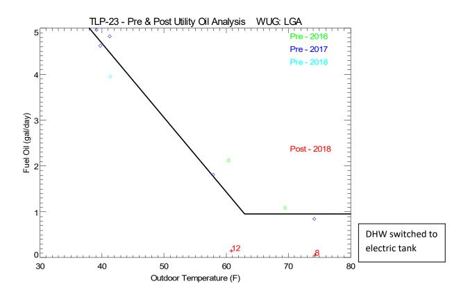
Figure 6. Trend of Oil Use with Outdoor Temperature Data, Using Fuel Delivery Logs from Pre, and Post-Retrofit Periods
