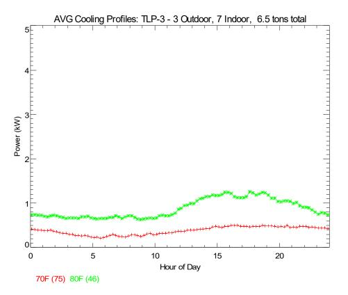
Figure 10. Heat Pump Demand Profile Across the Day – Averaged for Various Outdoor Temperature Bins (Cooling)
