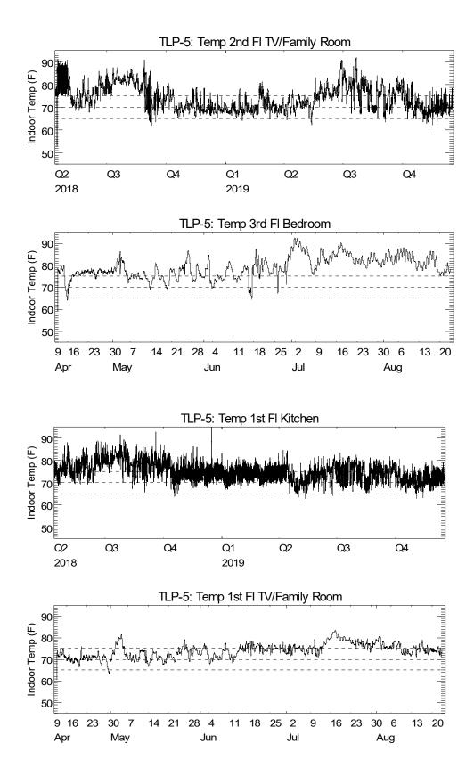
Figure 10. Plot of Space Temperatures at Various Indoor Locations
