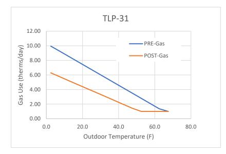
Figure 7. Trend of PRE- and POST-Retrofit Gas Use with Outdoor Temperature for Bin Analysis
