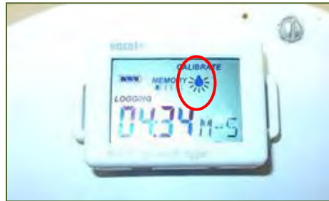
Figure 4: Light On - Bulb On
