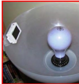
Installed with light sensor facing away from the bulb.
