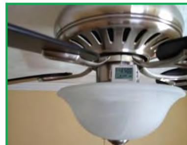
Attached by magnets with light sensor pointed down toward the bulb
