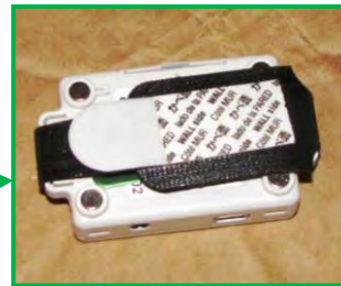
This is a curved recessed fixture – logger is installed using a 3M strip on the Velcro strap to stick to the curved surface
