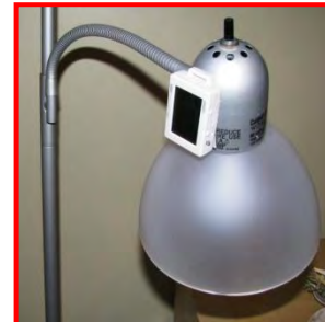
Logger is not focused in on any light source.
