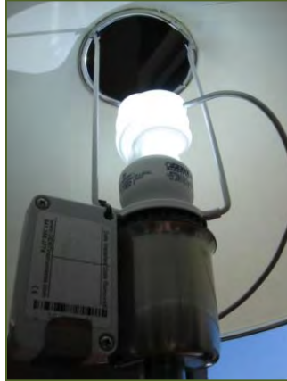
Figure 6: Fiber Optic Eye Aimed at Brightest Part of Light
