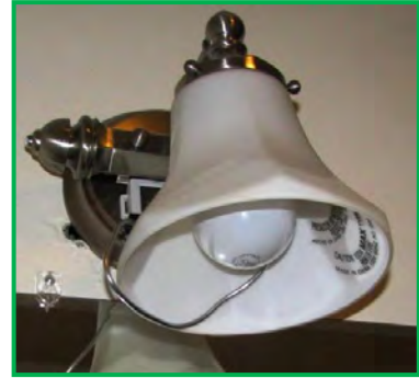
Logger is placed next to the fixture with a light pipe curving around fixture to focus directly on the light source
