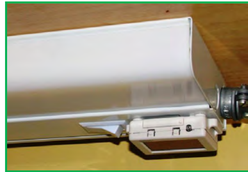
Logger is placed with the light sensor facing the light source.
