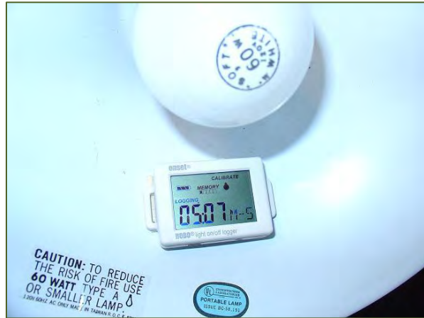
Figure 12: Logger Secured in Lamp with Command Strips
