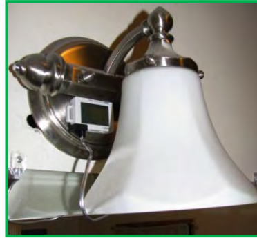
Logger is placed next to the fixture with a light pipe curving around fixture to focus directly on the light source
