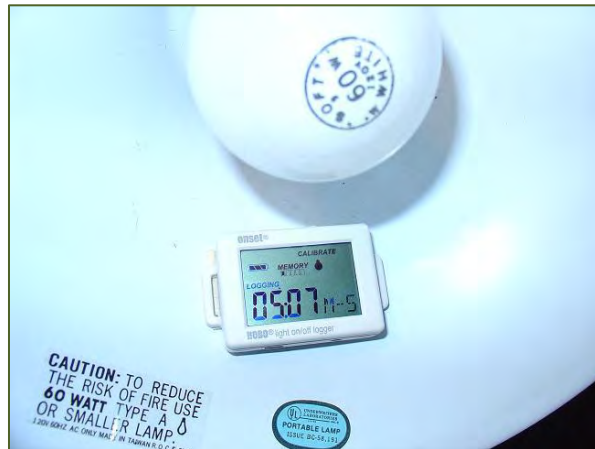
Figure 12: Logger Secured in Lamp with Command Strips
