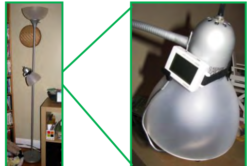
Logger is attached with the Velcro strip and uses a light pipe to focus in on the source.
