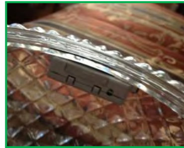
Logger is installed inside the lip of the light cover without being too visible to the homeowner.
