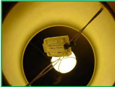
Logger is attached to lamp shade with zip ties with the light sensor facing the bulb.
