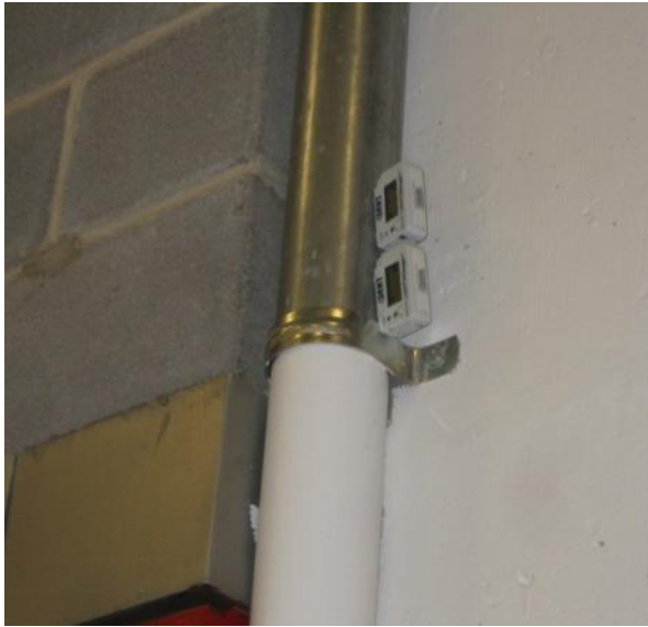
Figure 3-20. Installation of Lighting Loggers in Project #3, Energy-Efficiency Program Area
