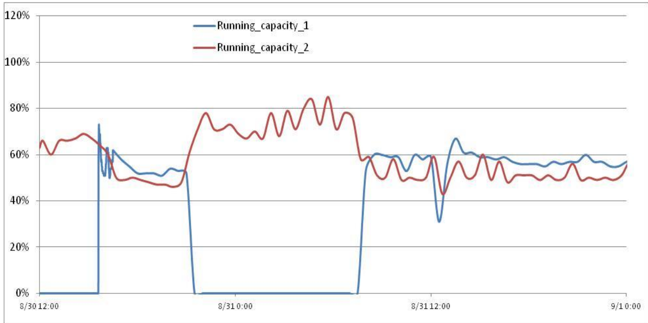
Figure 3-16. Chiller Capacity Trending at Project #2, Energy-Efficiency Program Area
