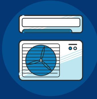
Air source heat pumps extract heat from outside air that is then used for heating indoor spaces during the colder months. They can also extract heat from indoors and expel it outside to cool indoor spaces during the warmer months. Air source heat pumps can be used to heat or cool single rooms (partial load) and whole homes (full load).
