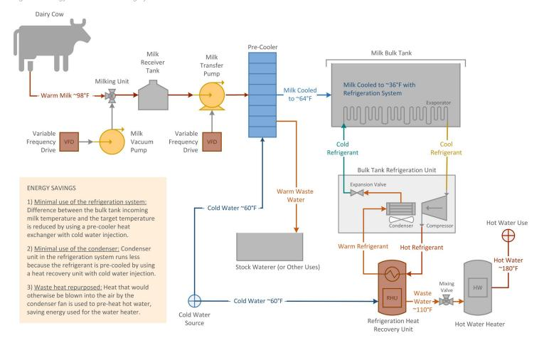
Figure 3. Energy-Efficient Milk Cooling System.
