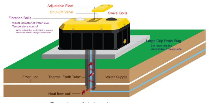
\*To prevent your vertical water supply line from freezing, an insulated thermal earth tube is installed under the ground during set-up.
