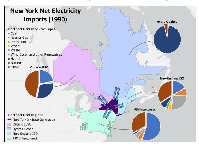
Figure 8. New York State Imported Electricity in 1990: Resource Mix Profiles and Regions
