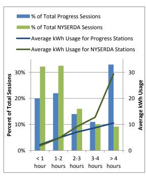
Figure 1: Energy Use and EVSE Comparison Between Progress Energy and NYSERDA Stations
