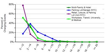
Length of Time With a Vehicle Drawing Power Per Charging Event (hr) max Range of EVSE Port Utilization avg min Multi-Family & Hotel
