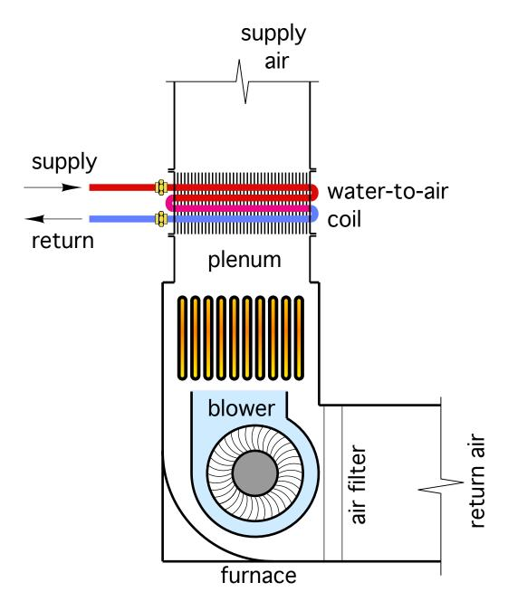
• Mounting the coil on the inlet of the furnace can cause the blower motor to overheat, leading to shutdown or burnout.
