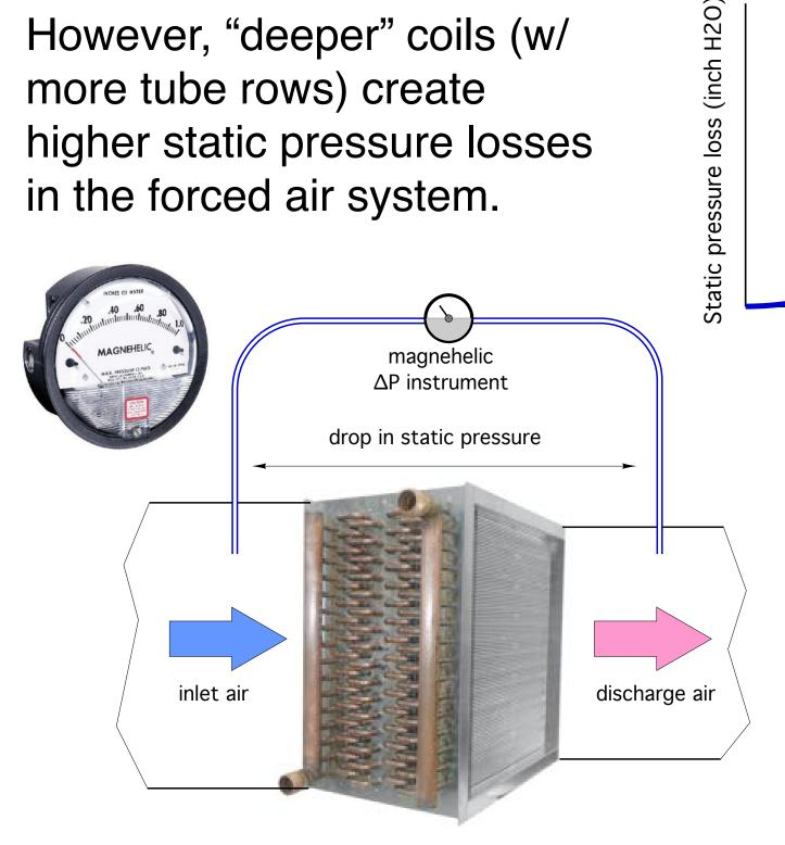
air flow rate (CFM) Get  $\Delta P$  vs. air flow rate data for specific coil from manf.
