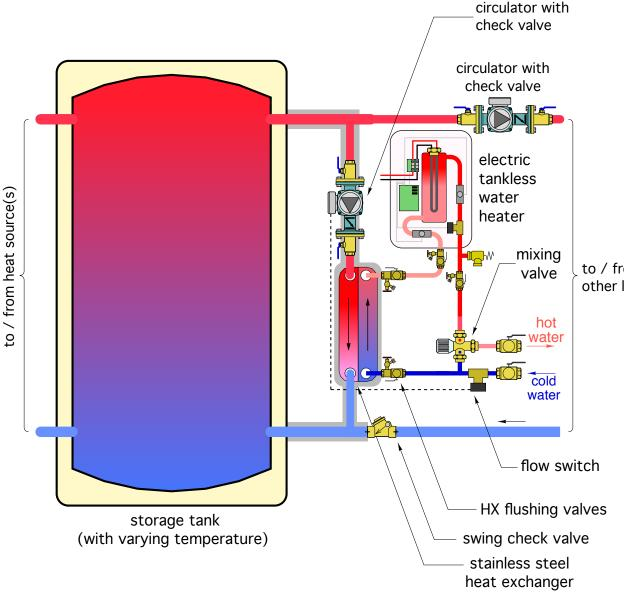
Electric water heater is thermostatically controlled to provide necessary temperature boost.
