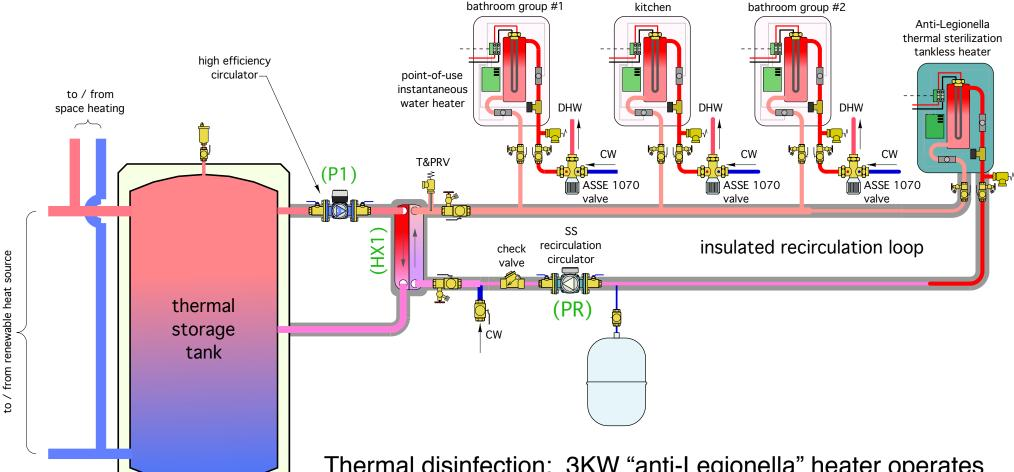
Thermal disinfection: 3KW "anti-Legionella" heater operates once per day to elevate DHW loop temperature to 140 °F for 30 minutes. This cycle is typically at night.
