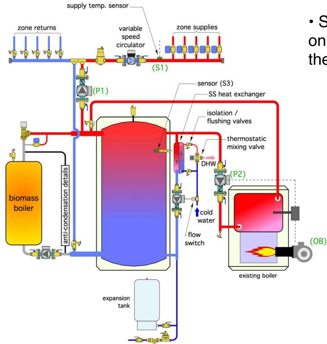
Supplemental boiler only heats top of thermal storage tank
