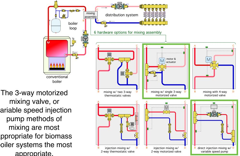
mixing valve, or variable speed injection pump methods of mixing are most appropriate for biomass boiler systems the most appropriate.
