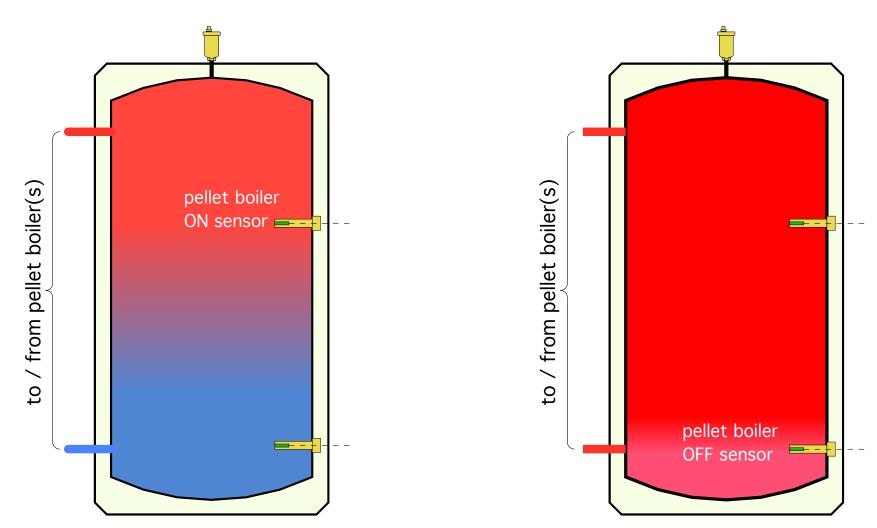
Pellet boiler fired when UPPER tank sensor drops to the target temperature of the outdoor reset controller Pellet boiler turned off when LOWER tank sensor climbs to some higher setpoint temperature.
