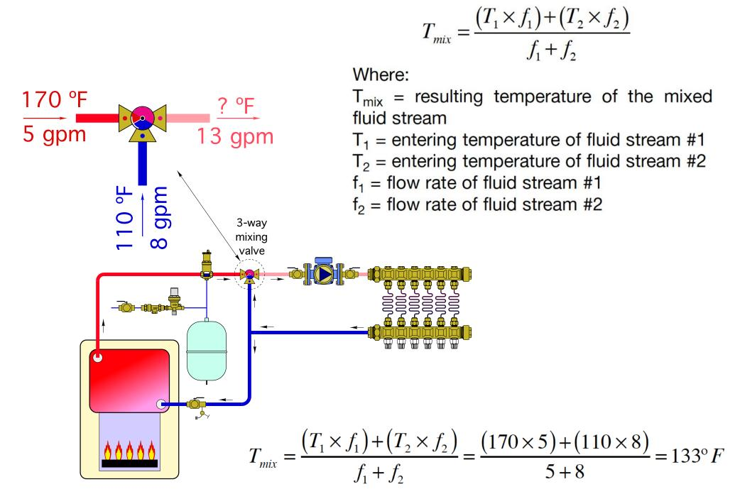
A mixing assembly is a collection of hardware components and control logic that regulates the rate of heat transfer from the heat source to the distribution system.
