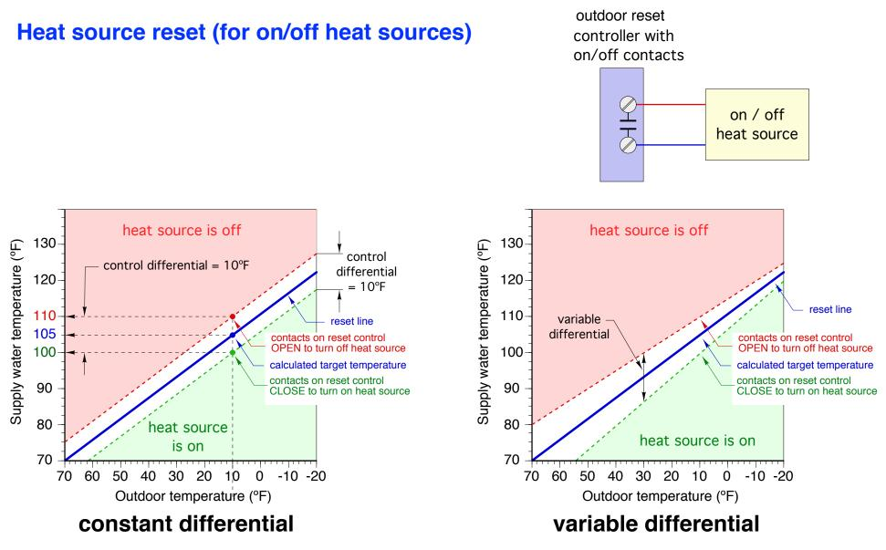
Design tip: Variable differential can reduce short cycling in systems with low mass heat sources.
