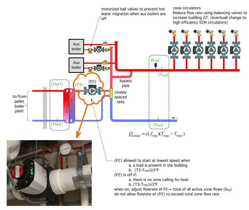
High efficiency ECM Circulators all have several speed control options such as 0-10VDC, 4-20ma, PWM, BACnet, LonWorx
