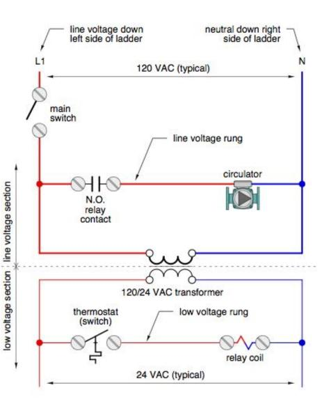
Two sections in a ladder diagram:
