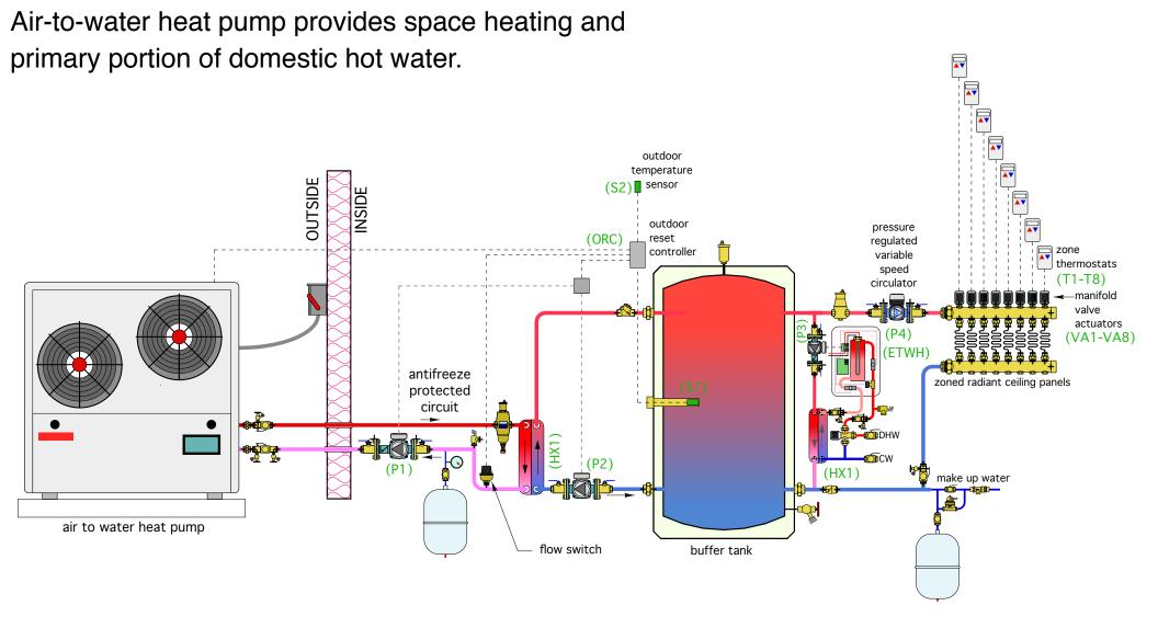
Design tip: Always make sure that all electrically powered components have the same designator in the piping schematic and ladder diagram.
