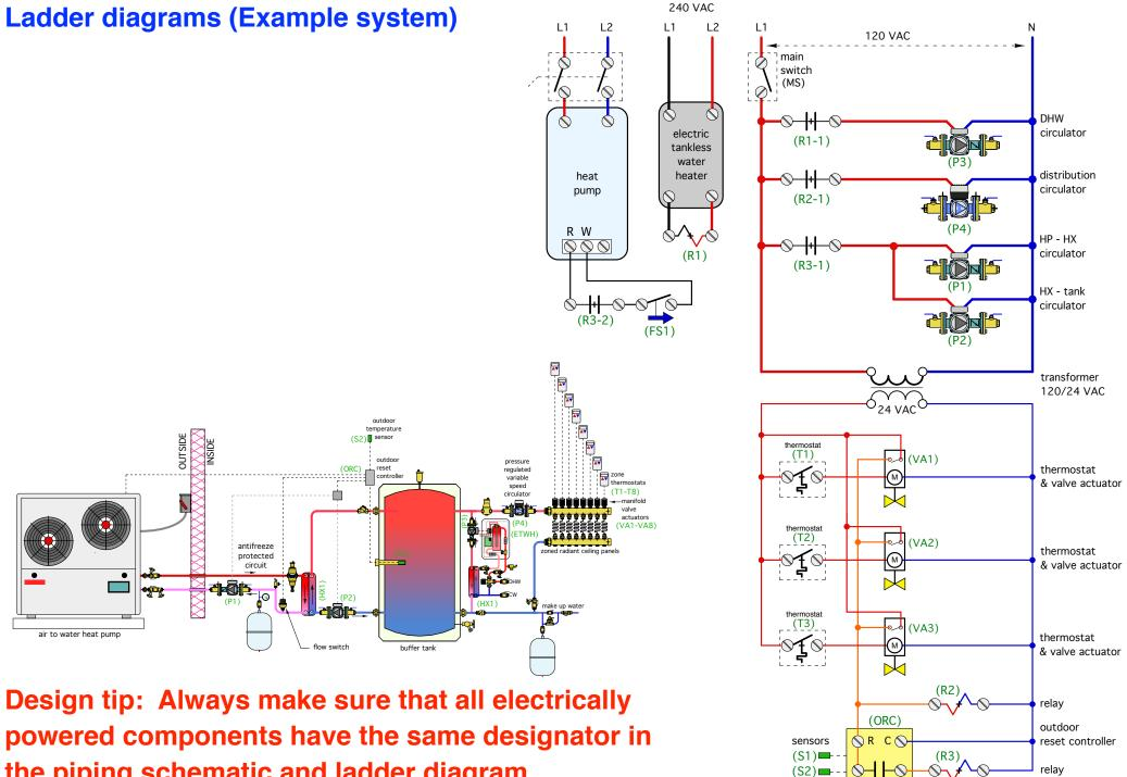
the piping schematic and ladder diagram.
