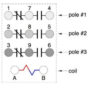
Design tip: I like a 3PDT relays from W.W.Graingers (5X840 w/ 24 VAC coil) (5X841 w/ 120 VAC coil) (5X853E socket) very versatile...
