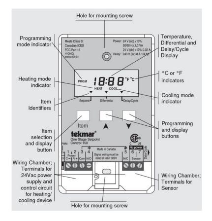
Design tip: Always check max sensor wiring distance, and use 18 ga copper twisted pair or shielded cable when running long distances (minimizes electrical noise interference)
