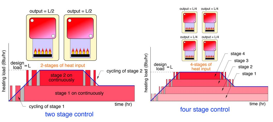
In theory, the great the number of stages, the better the ability to match heat output to load. However, the cost of the installation also increases with increasing number of stages.
