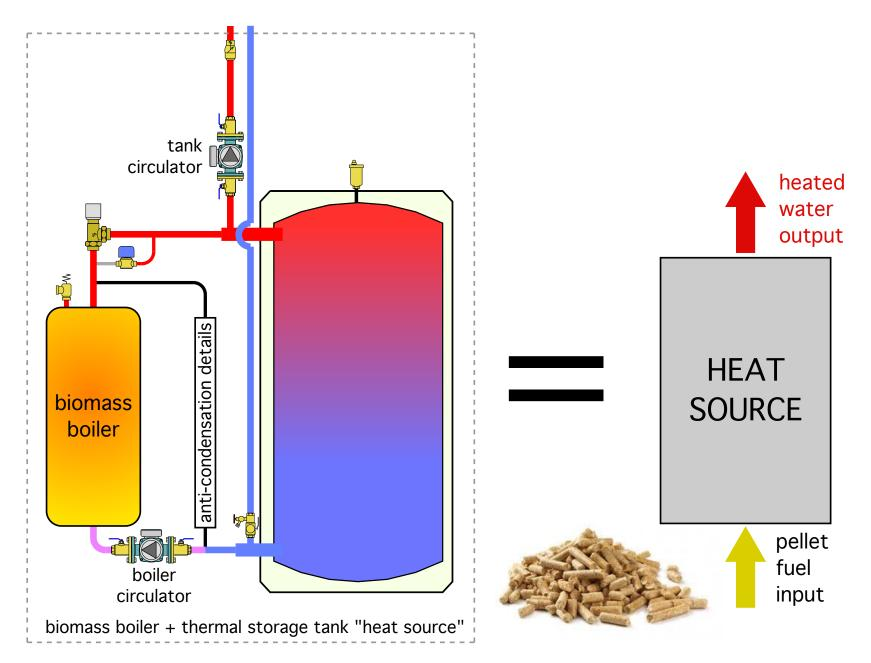
It's "intuitive" for designers to create systems where the biomass boiler is treated as a "fixed lead" stage, and the auxiliary boiler is the "lag" stage.
