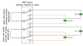
switch in one position routes (STU) & (STL) to boiler terminals label this position as "tank sensors control pellet boiler"
