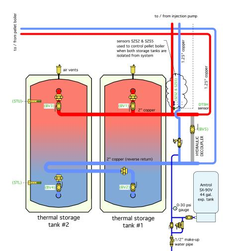
1. BOTH THERMAL STORAGE TANKS IN OPERATION: Valves (BV1, BV2, BV3, BV4) all open Ball valve (BV5) closed upper and lower temperature sensor in tank #2 (STL, STU )control pellet boiler
