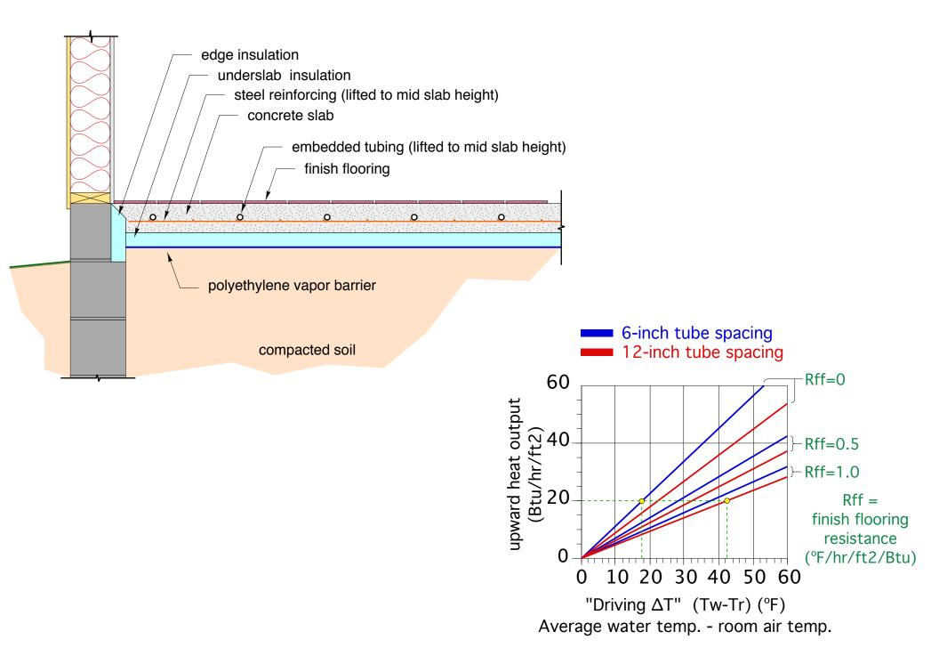
Distribution system: Examples of low temperature radiant panels
