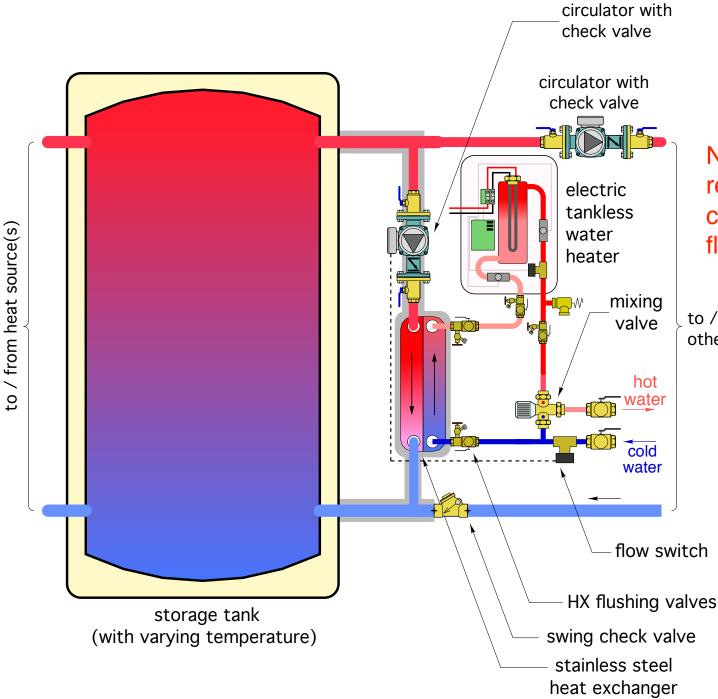
NOTE: Check valve required on tank-to-HX circuit to prevent reverse flow during space heating
