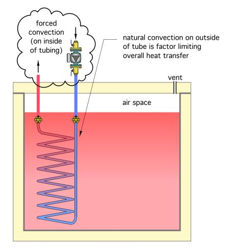
• For a given rate of heat transfer, the surface area associated with natural convection is much larger than that required by forced convection.
