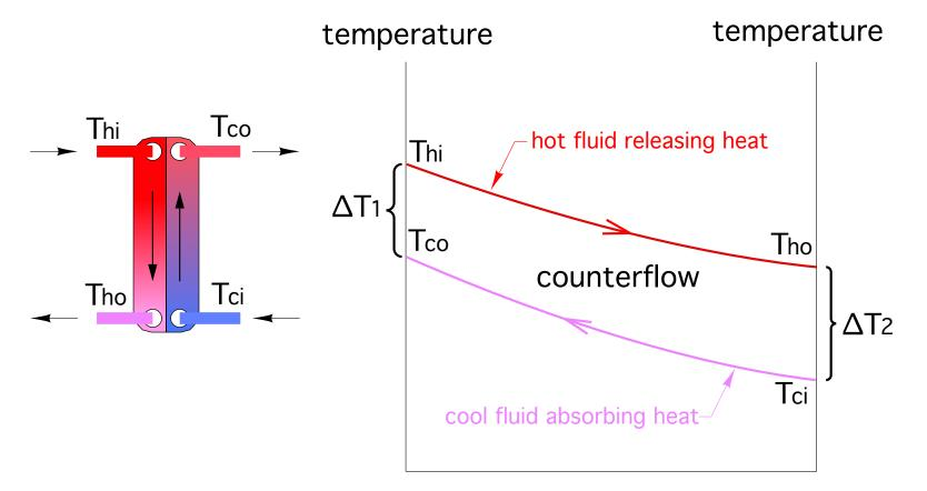
Counterflow ALWAYS produces the highest "log mean temperature difference" (LMTD) across the heat exchanger.
