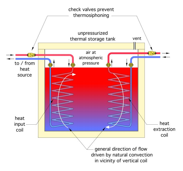
Limitations of internal coil heat exchangers
