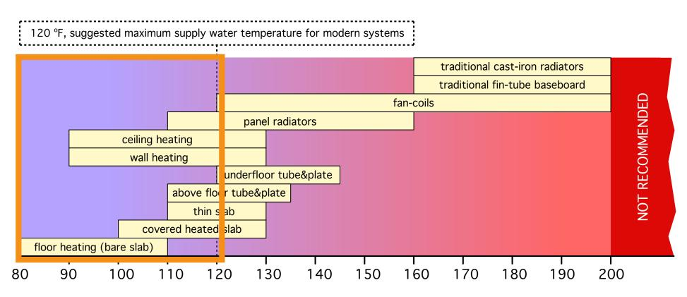
• Don't feel constrained to select heat emitters based on traditional supply water temperatures...
