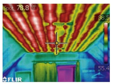
Thermal image of radiant ceiling in operation
