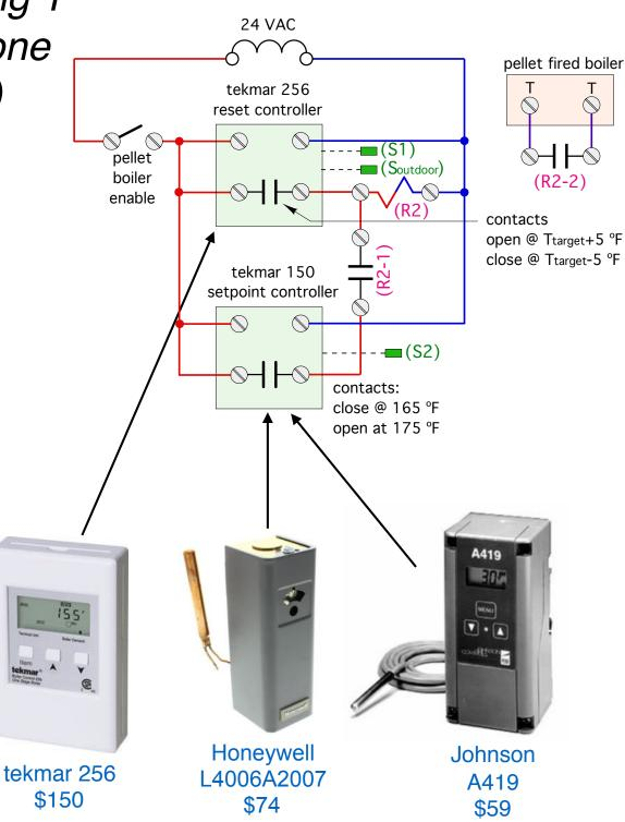
Adding *mixing* (based on outdoor reset) between the thermal storage tank and distribution system will smoothen heat delivery and significantly *improve comfort*.
