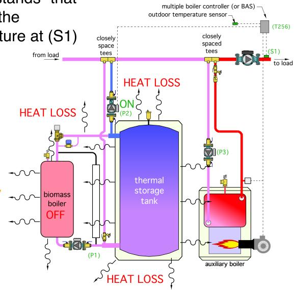
In a conventional multiple boiler system the added heat loss created by flow of heated water through an unfired boiler - *while not desirable* - doesn't create substantial heat loss:
