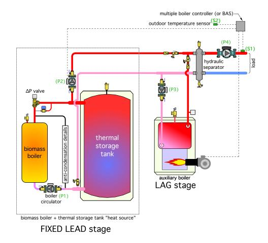
With this arrangement <u>(and proper controls)</u> energy added by aux boiler can be kept out of thermal storage. Assuming (P2) flow rate  $\leq$ (P4) flow rate, the coolest water is returned to the lower tank connection.
