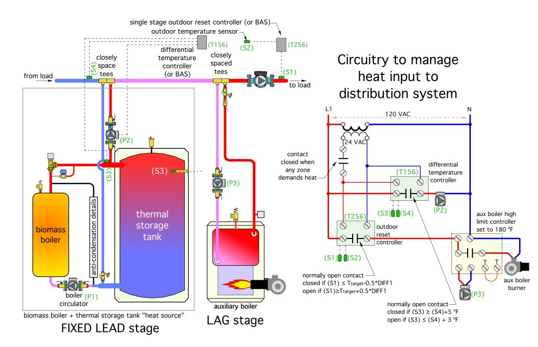
Using two simple, inexpensive controllers to manage heat flow to load
