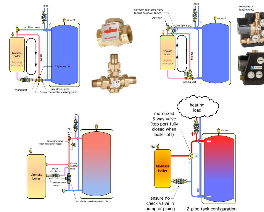
Think of the pellet boiler, combined with thermal storage as a "heat source" device
