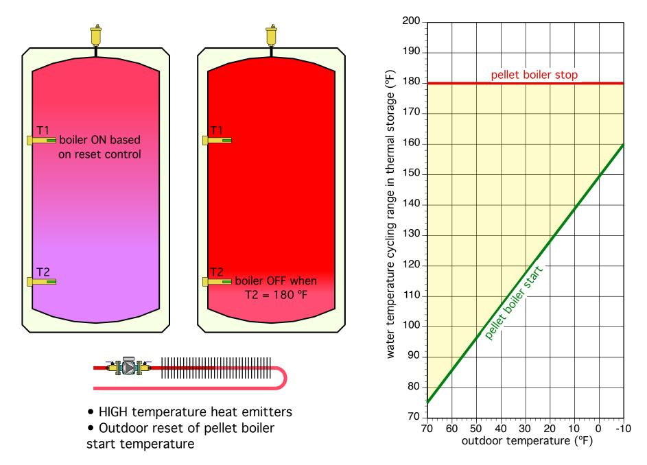
Temperature stacking *(using 1 setpoint temperature and one outdoor reset temperature)*
