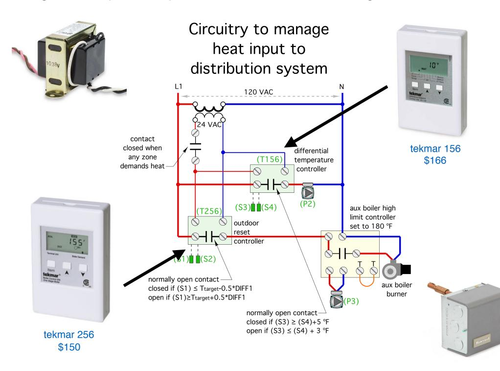
The same control concept can be applied to a system using a cordwood gasification boiler & auxiliary boiler
