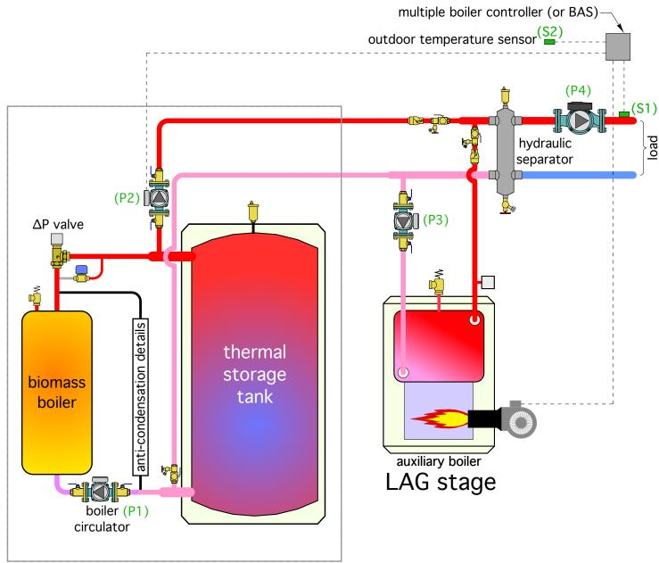
biomass boiler + thermal storage tank "heat source"
