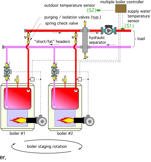
It's "intuitive" for designers to create systems where the biomass boiler is treated as a "fixed lead" stage, and the auxiliary boiler is the "lag" stage.
