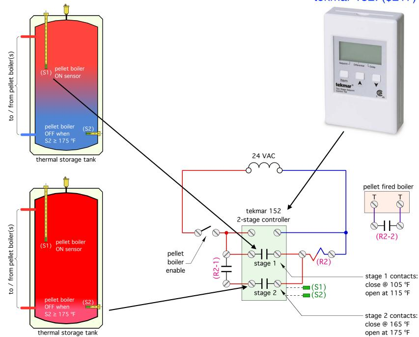
Temperature cycling range of storage is high dependent on the type of heat emitters used.
