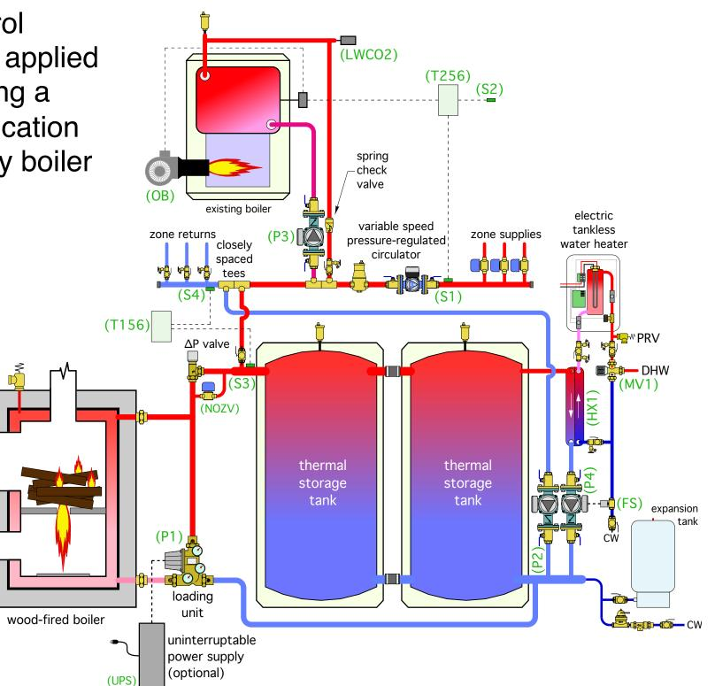
The same control concept can be applied to a system using a cordwood gasification boiler & auxiliary boiler
