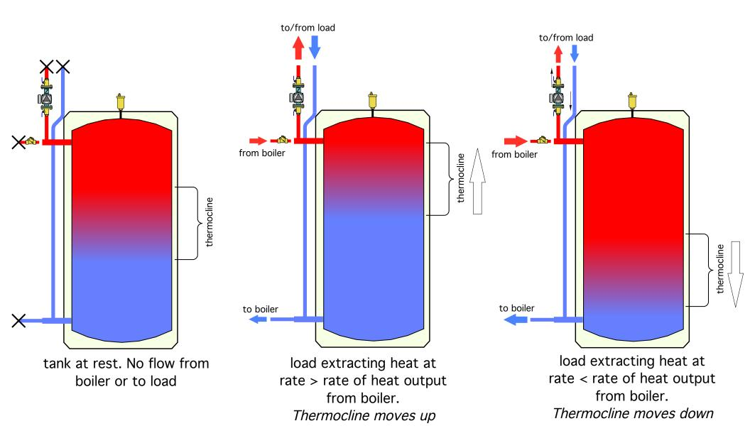
The pellet fired boiler should be turned on *before* the hot water is depleted from top of tank.
