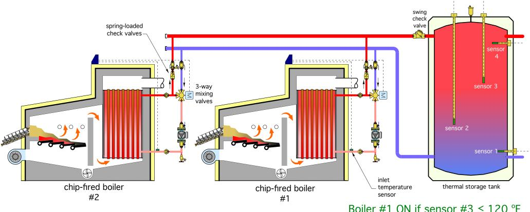
Firing order of boilers is periodically changes to help equalize boiler operating hours.
