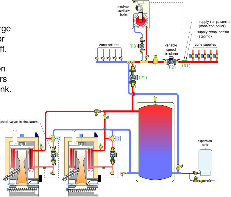
individual 3-way motorized valves for anti-condensation protection
