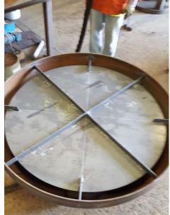
Baffle plate being welded into tank head & base shell at Troy Boiler Works
