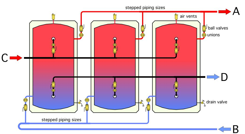
If using this piping be sure to plan for possibility of individual tank isolation and removal.
