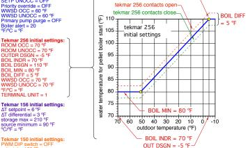
PWM DIP switch = OFF setpoint = 168 °F differential = 4 °F heat/cool = heat
