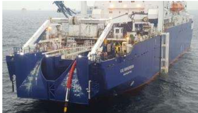
Figure 11.3-12 Inter-array Cable Installation Vessel
