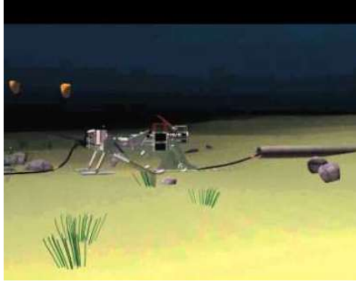
Figure 11.3-10 Indicative Picture of a Plow Burying a Cable
