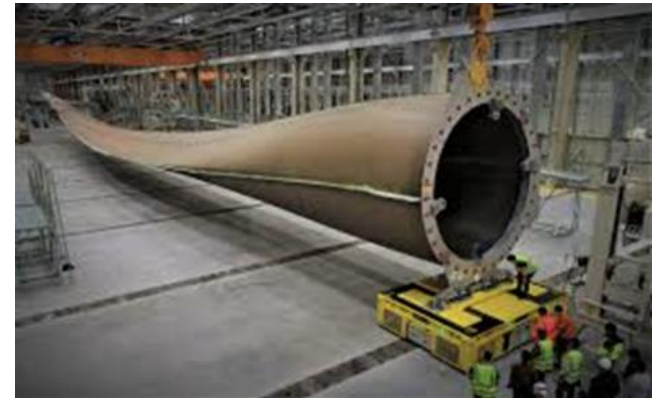
GE 12-MW Wind Turbine Nacelle (above) and 107-m Blade Below)
