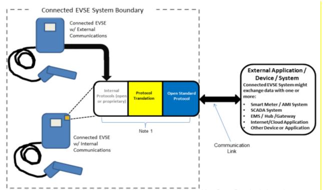
Note: Communication device(s), link(s) and/or processing that enables Open Standards-based communication between the EVSE and external application / device / system(s). These elements, either individually or together, could be within the EVSE, and/or an external communication module, a hub/gateway, or in the Internet/cloud.
