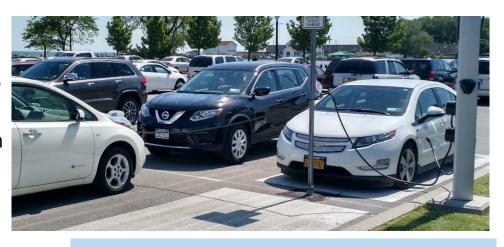
EVs have a portable charging cord that plugs into a 110V outlet and a site could provide only outlets for use by these portable cords as a very low cost option. However, EV charging outlets must be on a dedicated circuit and three-prong outlets will experience wear from everyday use (the EV connector was specifically designed for this).
