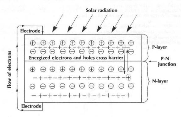
**Cross Section Diagram of a Photovoltaic Cell**
