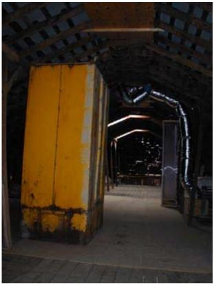
Figure 9. The vacuum equipment for the picker, in the upstairs loft of the barn.
