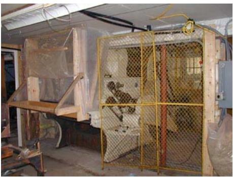
Figure 3.. Side view of picker exit, where wool is collected after it has been "picked" clean of any vegetable matter that remained after washing.
