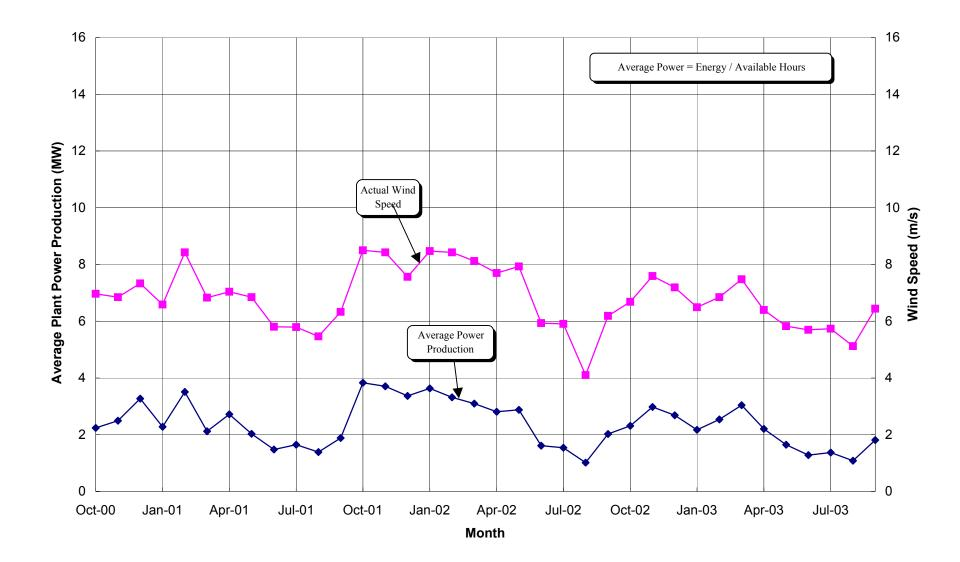
Figure 5-2: Monthly Mean Wind Speed and Average Plant Power Production -Madison Windpower Project-
