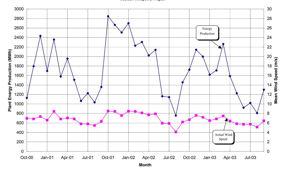
Figure 5-1: Monthly Mean Wind Speed and Plant Energy Production -Madison Windpower Project-
