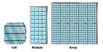
**Figure 1.** Diagram that shows how individual cells make up a module. An array consists of sets of modules (from the National Renewable Energy Laboratory, Golden, CO).
