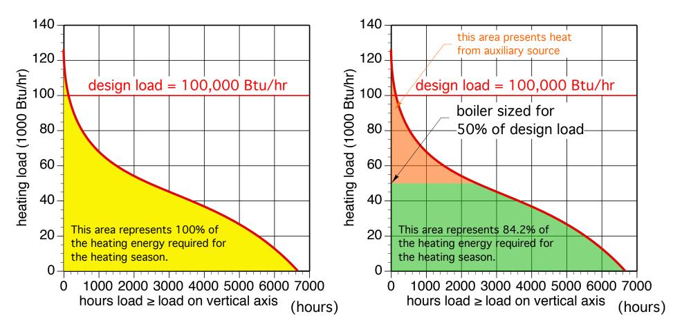
Boiler sized @ 50% of design load provides about 84% of seasonal space heating energy.
