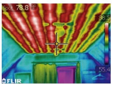
Thermal image of radiant ceiling in operation
