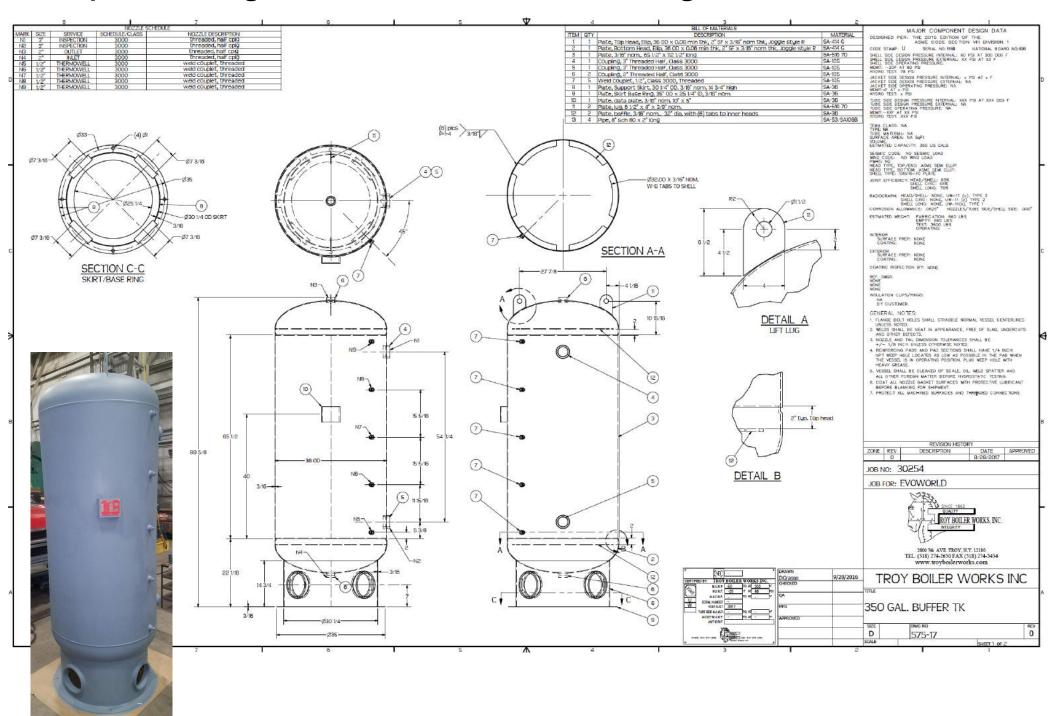
Large ASME (section VIII) certified storage tanks intended for domestic water heating are not necessarily a good choice for thermal storage in hydronic systems .
