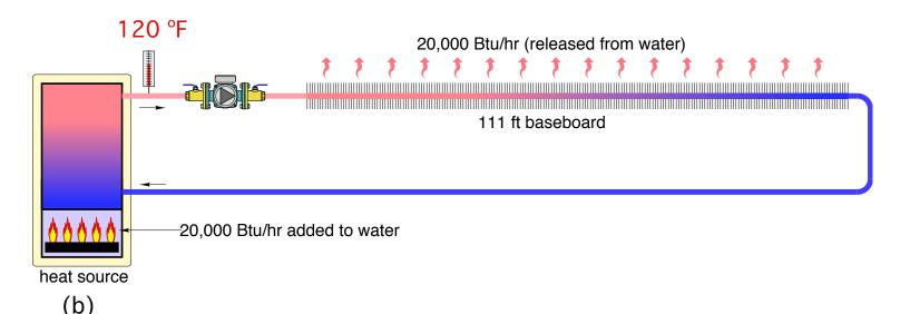
In retrofit applications the existing heat emitters and distribution system are likely to be sized based on relatively high supply water temperatures (180-200 °F) at design load conditions.
