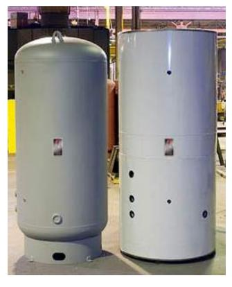
The connections are usually not in the right locations, or of the size needed for hydronic systems (and good temperature stratification).
