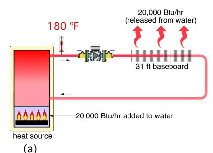
The greater the linear footage of baseboard, the lower the supply water temperature requirement.
