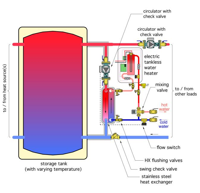
• Leverages the thermal mass for stabilizing DHW delivery.
