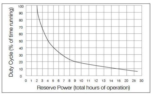
Performance curve results using a 3/4 HP pump with a 7.5 FLA and (2) Metropolitan Power Plus model 31P-36 batteries.
