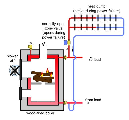
It's necessary to protect wood-fired boilers from low entering water temperatures.
