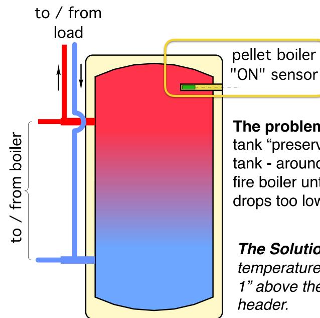
**The problem:** Stratification within tank "preserves" hot water at top of tank - around sensor - and fails to fire boiler until water temperature drops too low.
