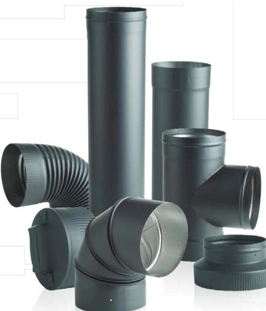
Secure all joints in single wall vent connector piping with <u>stainless steel</u> <u>sheet metal screws.</u>  Seal joints with high temperature (1000 °F rated) black silicone sealant
