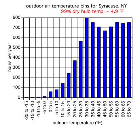
Figure 6-19. Frequency and range of outdoor temperature for a typical year in Syracuse, NY
