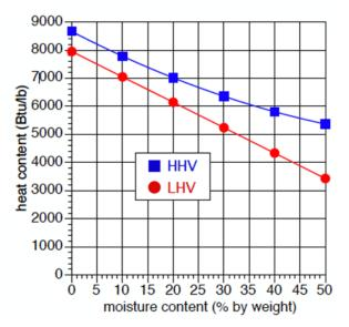
The maximum moisture content of cordwood used in a cordwood gasification boiler is 20%, even drier cordwood is preferred. Reducing split cordwood to a moisture content of 20% or less generally requires storage with open air circulation and protection from precipitation for at least one year.
