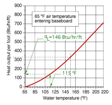
Figure 6-12. Determining the value of qL for an average circuit water temperature of 115°F
