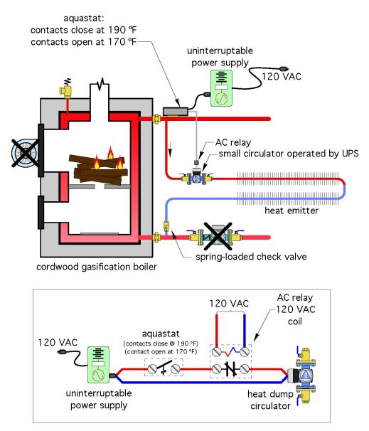
Note that an aquastat is installed on the piping near the boiler outlet. Its electrical contacts close whenever the boiler outlet temperature is at or above a value at which heat dissipation during a power outage should be in effect. These contacts open at a lower temperature where heat dissipation is not necessary. The aquastat limits heat dump operation to situations where the boiler is at an elevated temperature, and thus conserves battery power within the uninterruptible power supply.
