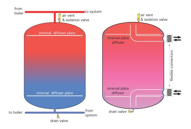
Figure 5-14. Cut away illustration of upper and lower plate diffusers combined with piping options
