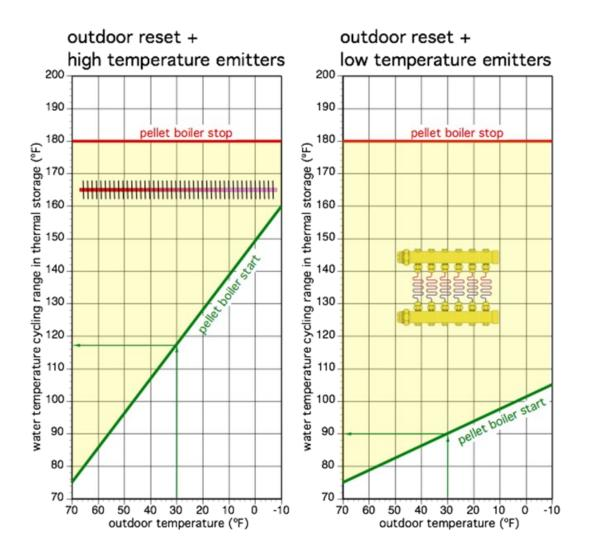
Under design load conditions the high-temperature system starts the pellet boiler when the thermal storage temperature drops to 160°F. At the same outdoor temperature condition, the low-temperature system starts the pellet boiler when the tank temperature drops to 105°F. The low-temperature system provides a much wider temperature cycling range at design load conditions.
