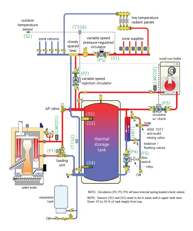
Note: Sensor (S5) should be mounted in the same well as sensor (S3). That well should be 10–20% of the tank height down from top.
