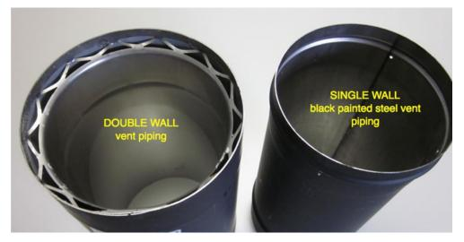
Twenty-two gauge, black-painted, single-wall stove pipe is available from many suppliers in a range of sizes and with associated fittings such as elbows, tees, and caps. This pipe is swaged on one end, allowing sections to be joined without crimping. The swaged end of the pipe should always be installed up, to allow any condensate within the pipe to remain within the pipe as it drains downward.
