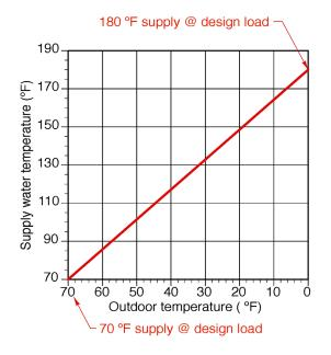
Outdoor reset can be very useful in extending the temperature cycling range of thermal storage tanks used in biomass boiler systems under partial-load conditions. Figure 6-21 shows an example.
