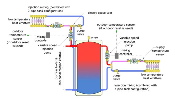
The variable speed pump can be a standard wet-rotor circulator with a permanent split capacitor (PSC) motor or a circulator with an electronically commutated motor (ECM).
