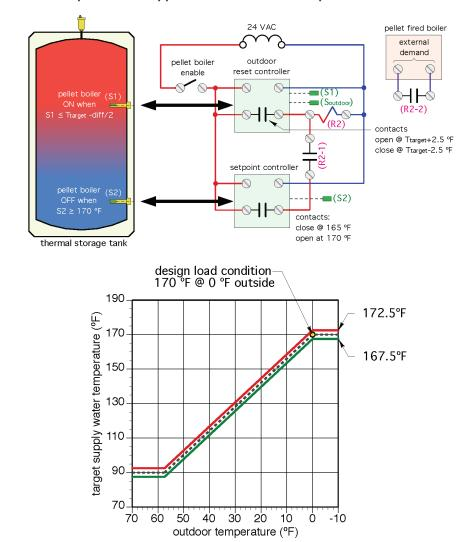
Figure 7-15. Electrical schematic for the two-sensor method of turning a pellet boiler on and off. Graph shows water temperature at upper tank sensor at which pellet boiler turns on.
