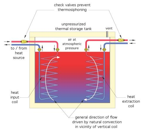
The coil on the left delivers heat from the biomass boiler to the tank. Water inside this coil flows from top to bottom, as tank water rises due to buoyancy as it absorbs heat. The coil on the right supplies heat from the tank to the load. Water within this coil flows from bottom to top as water in the tank descends due to increasing density as the water cools.
