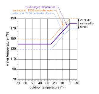
Figure 8-4c. Outdoor reset controller settings for (T256) controller in system 4
