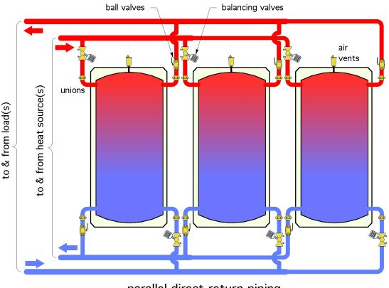
Figure 5-25. Three thermal storage tanks piped in parallel direct-return configuration
