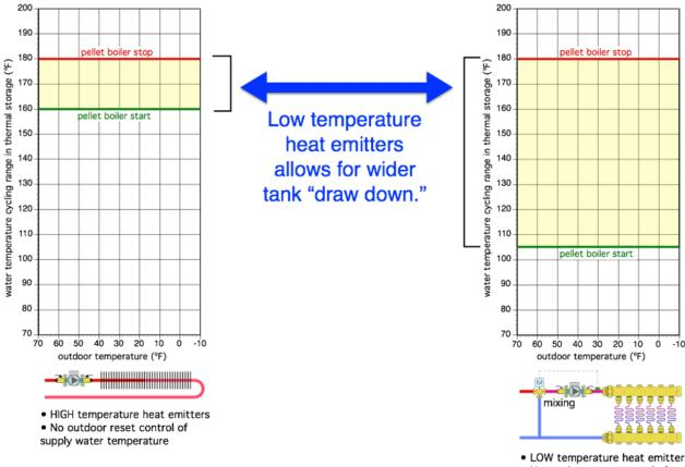
Figure 3-4. Comparison of temperature cycling range for a thermal storage tank using high-temperature heat emitters versus low-temperature heat emitters
