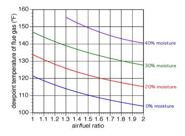
The air/fuel ratio is the ratio of the amount of air supplied to the combustion process divided by the "stoichiometric" minimum amount of air needed to completely burn the fuel. Supplying excess air to the combustion process creates a drying effect that lowers the dewpoint of the flue gases. However, as more air is supplied more heat is carried away in the exhaust stream.
