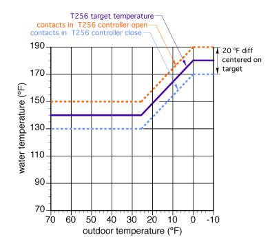
Figure 8-5c. Setting the outdoor reset controller (T256) in system 5
