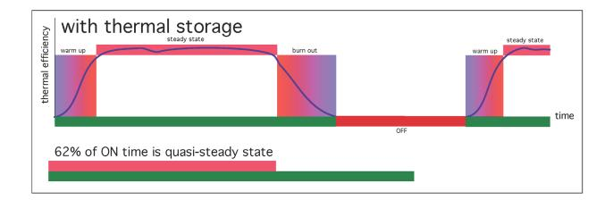
Figure 3-1 shows the percentage of elapsed time the boiler operates at or close to steady state combustions conditions. The scenario with longer and less frequent boiler cycling yields a higher percentage of quasi-steady state combustion. The higher this percentage, the higher the overall integrated efficiency of the boiler and the lower its emissions.
