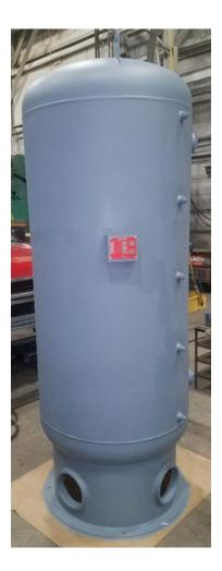
The tank is 35 inches in diameter and approximately 100 inches tall, and weighs about 660 pounds. The tappings seen on the side of the tank are used for mounting temperature sensor wells. It has two, three-inch FPT tappings near the top and bottom of the cylindrical shell, as well as a two-inch FPT tapping at the very top and bottom of the tank. The metal primer finish prevents surface oxidation.
