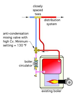
Figure 7-22. Auxiliary/existing boiler piping that includes an anti-condensation thermostatic mixing valve
