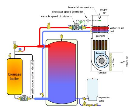
Ideally, the water-to-air heat exchanger coil should be selected to provide design load heat output using a water temperature no higher than 120°F. Doing so allows a wide temperature cycling range within the thermal storage tank and helps ensure long on-cycles for the biomass boiler. This suggested temperature limit of 120°F for the coil will likely require it to have multiple tube passes, such as shown in Figure 7-32.
