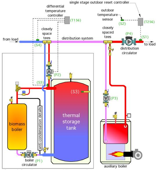
Figure 7-24. Differential temperature controller (T156) combined with an outdoor reset controller (T256) and their associated temperature sensors
