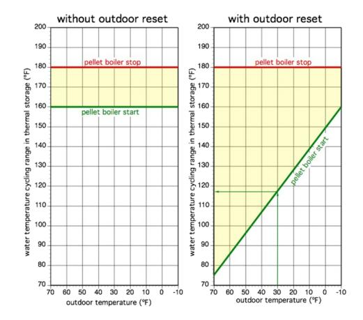
Figure 6-21. Comparison of water temperature cycling range in thermal storage based on systems with and without outdoor reset of the water temperature supplied to the heat emitters
