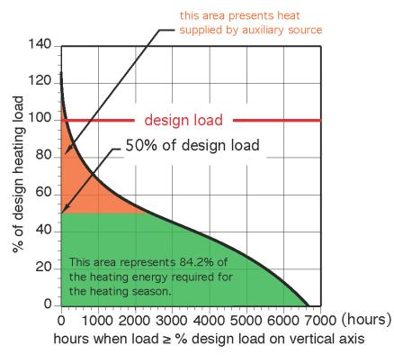
The green shaded area shows that 84.2% of the total seasonal heating energy use occurs when the heating load is 50% or less of design load. The remaining 15.8% of seasonal energy use occurs when the heating load is greater than 50% of design load. This implies that a boiler sized to 50% of design load could supply about 84% of the total seasonal heating energy requirement.
