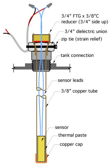
The length of the well can be whatever is required. This is helpful when a sensor needs to be located at a specific height in the tank, and the well needs to be mounted from the top of the tank. Be sure there's adequate head room to insert the well. If not, mount the well in the tank before the tank is positioned.
