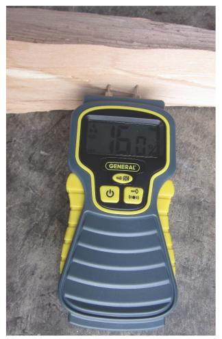
Proper assessment of the average moisture content of stacked cordwood should be based on measurements from several pieces taken from different areas of the stack. The end-grain moisture content along with the moisture content of internal fibers (wood samples are split open) should be measured. It's common for cordwood to have significantly higher internal compared to end-grain moisture content.
