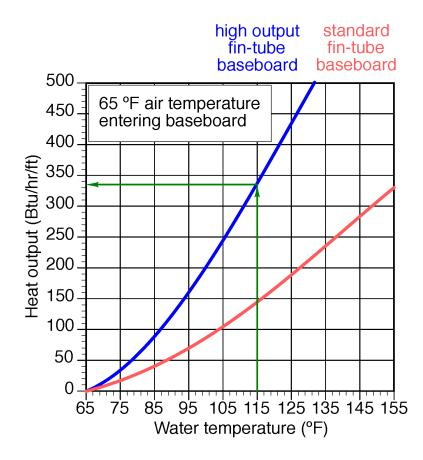
The steps of the previous procedure can be modified to determine the amount of high-output, finned-tube baseboard that is required to reduce the supply water temperature to the system under design load.
