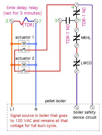
The damper actuators and the time delay relay (TDR) are energized as soon as a 120 VAC signal within the boiler turns on at the beginning of the combustion cycle. That signal source must provide a stable 120 VAC throughout the combustion cycle. A normally closed contact (TDR-1 NC) is wired in series with
