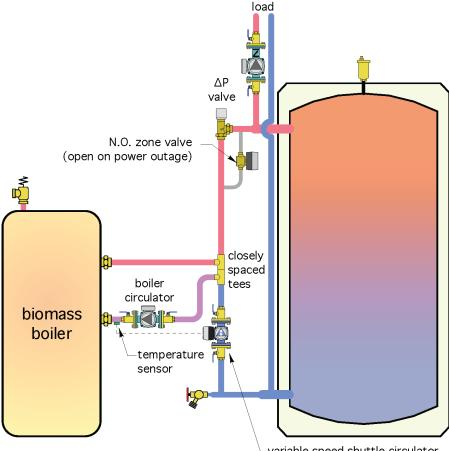
The boiler circuit consists of a short piping loop containing a fixed speed circulator. The tank circuit is another short piping assembly containing the variable speed shuttle circulator,  $\Delta P$  valve, and a normally open zone valve. The boiler circuit and tank circuit are coupled with a pair of closely spaced tees that hydraulically separate the boiler circulator from the variable speed shuttle circulator.
