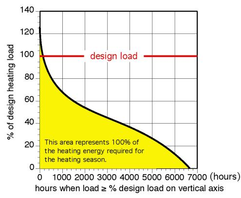
The vertical axis of this graph represents the percent of the design-heating load. The horizontal axis shows the hours during which the heating load is equal to or greater than the percent of design-heating load on the vertical axis. Although this graph is specific to the statistical weather data for Syracuse, NY, the characteristic curved shape of the shaded area is typical of other cool or cold climate locations.
