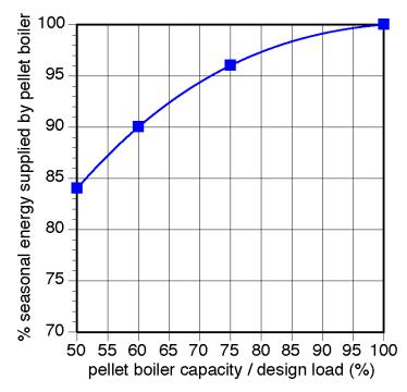
Figure 3-25 indicates that a pellet boiler sized to 75% of design load, in Syracuse, NY, could supply about 96% of the total seasonal space heating energy requirement. The remaining 4% would be provided by a supplemental heat source, such as another boiler, or other heating devices in the building.
