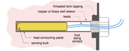
Figure 7-38. Illustration of the proper placement of a sensor in a well
