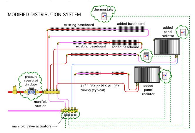
Figure 6-17. Distribution system using low-voltage manifold valve actuators on each circuit
