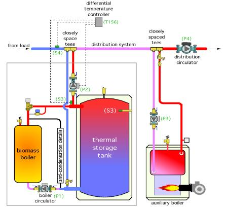
Figure 7-23. Placement of a differential temperature controller and its associated temperature sensors
