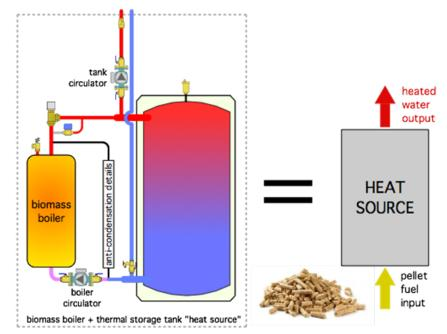
With a two-pipe or three-pipe tank configuration, heat flowing to the remainder of system is, at times, produced by the boiler, at other times it comes from storage, and sometimes from both at the same time. To emphasize the concept of the biomass boiler and thermal storage as a single heat-source entity, this combination will be referred to as biomass boiler + storage heat source.
