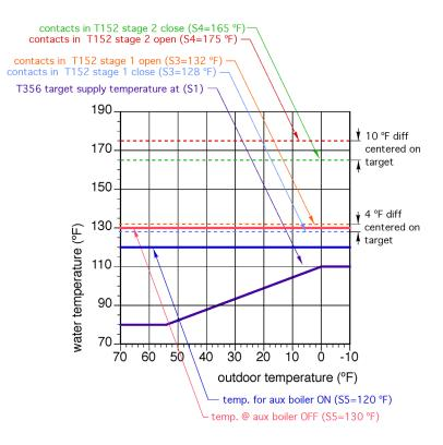
Figure 8-3c. Suggested controller settings for system 3
