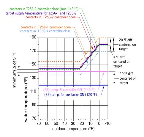
NOTE: The temperature at which the (T150-2) controller opens its contacts must be at least 3  $^{\circ}$  F lower than the lowest temperature at which the (T256-2) controller closes it contacts. In Figure 8-2c the (T150-2) controller opens its contacts at 140  $^{\circ}$  F. The lowest temperature at which the (T256-2) controller closes its contacts is 143  $^{\circ}$  F.
