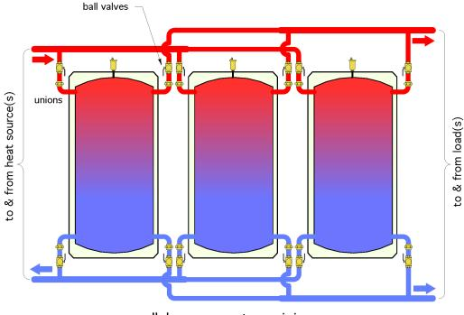
Figure 5-26. Three thermal storage tanks with a parallel reverse-return piping configuration
