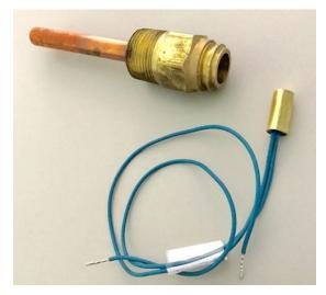
Before inserting the sensor, a small amount of thermal paste should be injected into the end of the well using a plastic syringe. The sensor body should also get coated with thermal paste. The objective is to completely fill the gap between the sensor body and inside surface of the well with thermal paste, as shown in Figure 7-38.
