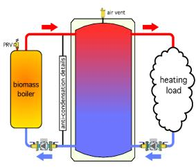
Figure 5-17. Four-pipe tank configuration connecting the biomass boiler and heating load
