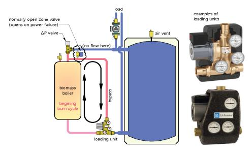
Figure 7-8. Loading unit installed between biomass boiler and thermal storage tank, and examples of loading units available in North America
