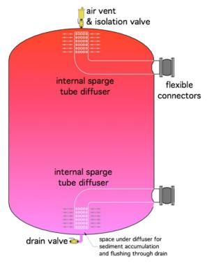
Sparge tubes have a closed end with a symmetrical array of holes around their perimeter. The total cross-sectional area of these holes should provide for low-average flow velocity.
