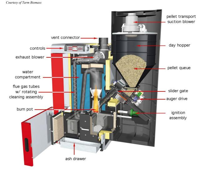
Figure 3-11. Cutaway of a pellet boiler with its associated day hopper
