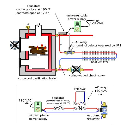
Figure 2-9. Piping and wiring for an active heat dump system
