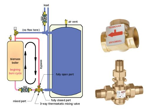
The mixing valve and bypass piping are installed between the biomass boiler and thermal storage tank. The boiler circulator must be installed between the mixing valve and the boiler, as shown in Figure 7-6.
