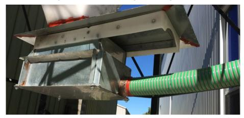
Figure 3-15. Flexible helical auger installed within a single-flexible guide tube
