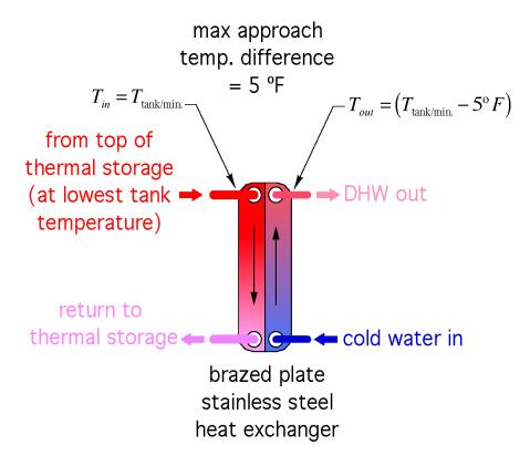
If the pellet boiler cannot maintain a sufficient temperature in the upper portion of the tank, the existing/auxiliary boiler operates based on the temperature at sensor (S3) in the upper portion of the thermal storage tank. The minimum temperature at sensor (S3) should be at least 5°F higher than the desired DHW delivery temperature.
