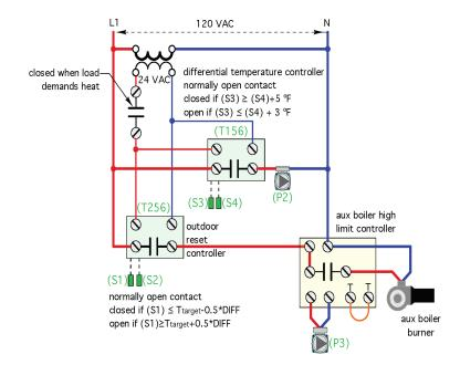
This circuitry assumes that the differential temperature controller (T156) and outdoor reset controller (T256) are powered by 24 VAC. That power only reaches both controllers when there is a heating demand in the system, which is evidenced by a closed relay contact. The latter is typically supplied from a multizone relay center or a thermostat if the building has only one zone.
