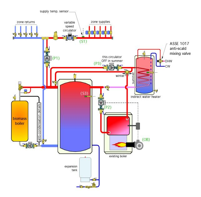
Figure 7-30. Integrating an indirect domestic water heater into a biomass heating system
