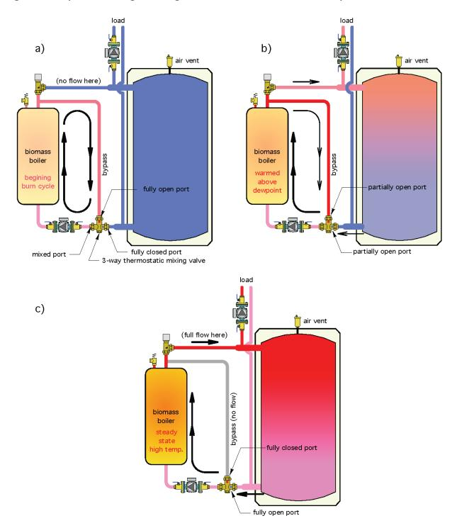
Figure 7-7. Sequence showing the changes in water flows as boiler water temperature increases
