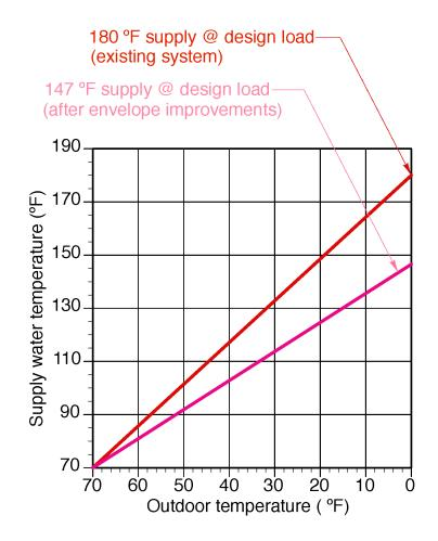
In this example, reducing the design heating load from 100,000 Btu/hr to 70,000 Btu/hr reduced the required supply water temperature under design load conditions from 180°F to 147°F. Although this is certainly an improvement, it is still substantially above the previously suggested design criteria of 120°F supply water temperature at design load.
