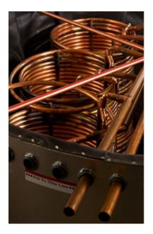
The thermal performance of coil heat exchangers is dependent on many variables including coil material, pipe diameter, coil height, diameter, flow rate, properties of the fluid flowing through the coil, and temperature stratification within the tank. Attempting to accurately calculate the theoretical heat transfer rates associated with natural convection can be very complex. For this reason, it is best to obtain heat transfer rate performance directly from the tank manufacturer.
