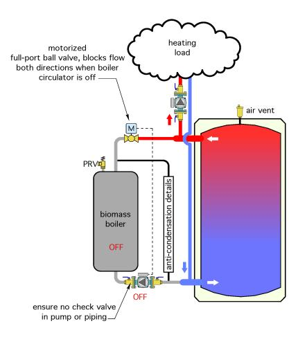
The motorized ball valve is wired in parallel with the boiler circulator. It opens as soon as this circulator turns on. Its spring-loaded actuator closes the valve as soon as the boiler circulator turns off. Use of a motorized full-port ball valve, with a high Cv value, minimizes head loss in the boiler circuit whenever the valve is fully open.
