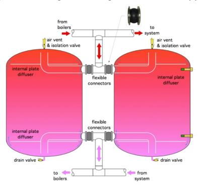
Figure 5-28. Configuration for two large thermal storage tanks that forms a two-pipe tank array
