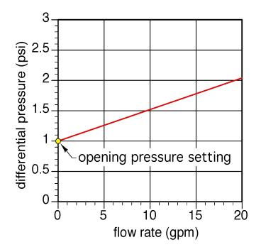
This characteristic allows the valve to have sufficient forward opening resistance, as well as maintains relatively low-head loss through the valve when the boiler circulator turns on. A differential pressure valve used in this manner closes as soon as the boiler circulator turns off. This prevents undesirable reverse thermosiphoning between the thermal storage tank and boiler. It also eliminates the need for a check valve in the boiler circuit.
