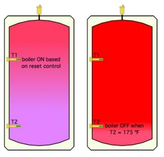
The upper sensor is used to turn the pellet boiler on when the temperature at that sensor drops to or below some "target" temperature that is continually calculated by the outdoor reset controller based on the outdoor air temperature.
