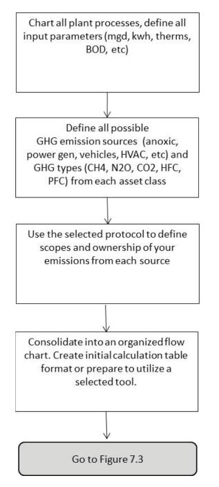
Figure 7.2 Conceptual flowchart for setting boundaries and identifying assets
