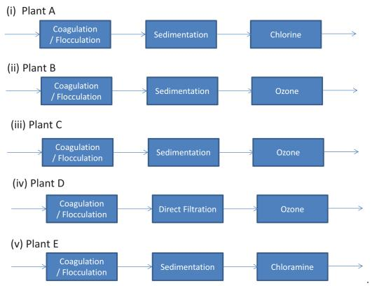
Figure 7.9 Conceptual process flow diagrams of the treatment plants
