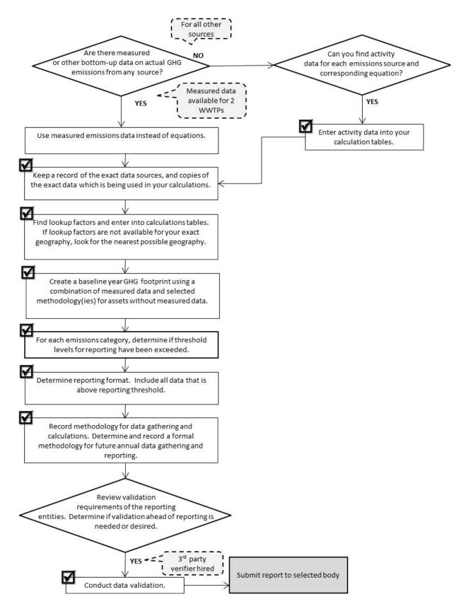
Figure 7.7 Data collection and reporting flowchart utilized by the wastewater case study
