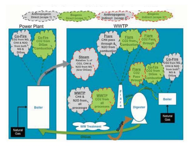
Figure 7.5 Sources of GHG Emissions from Large WWTP
