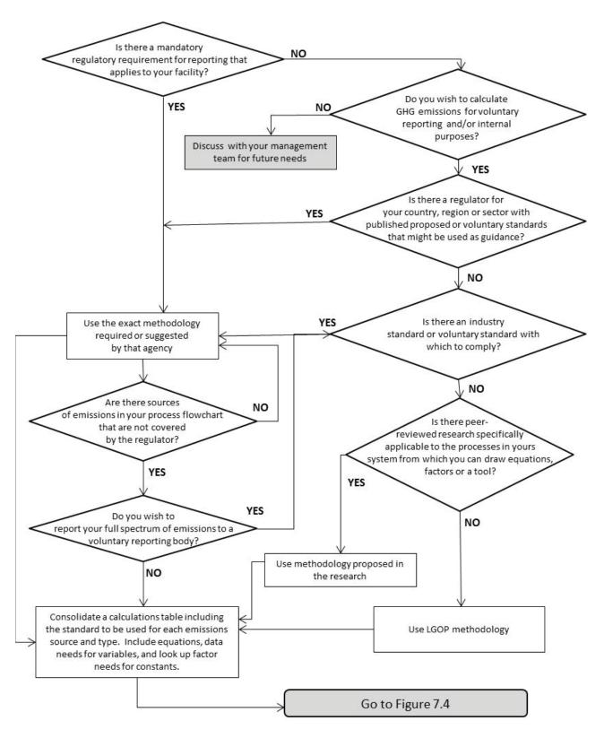
Figure 7.3 Flowchart showing protocol selection process
