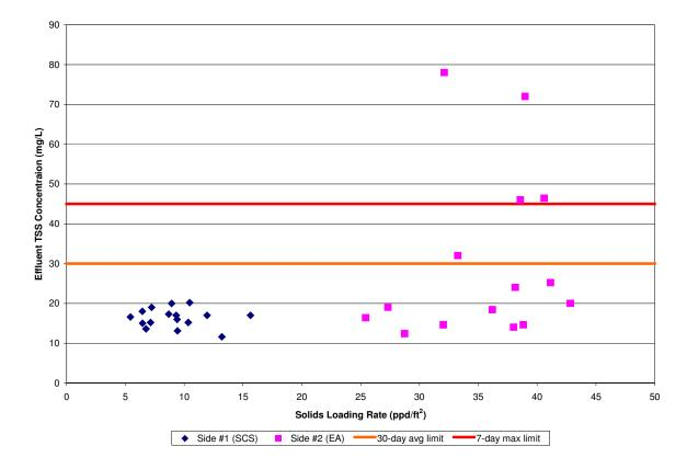
Figure 8-3. Effluent TSS Concentration versus Clarifier Solids Loading Rate
