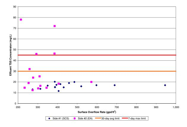
Figure 8-5. Effluent TSS Concentration versus Clarifier Surface Overflow Rate
