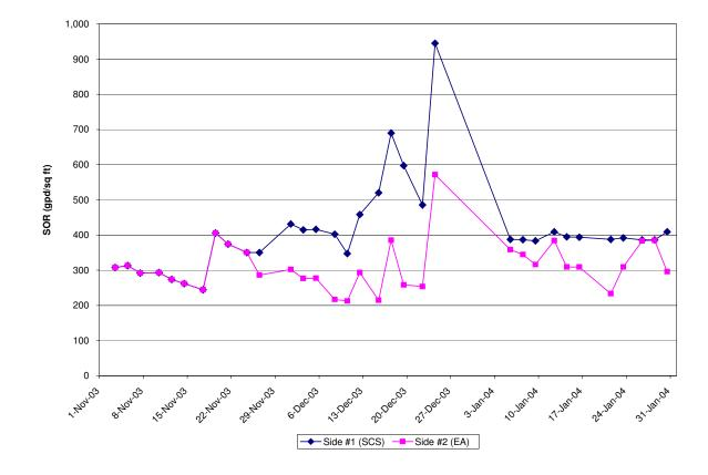
Figure 8-4. Clarifier Surface Overflow Rate
